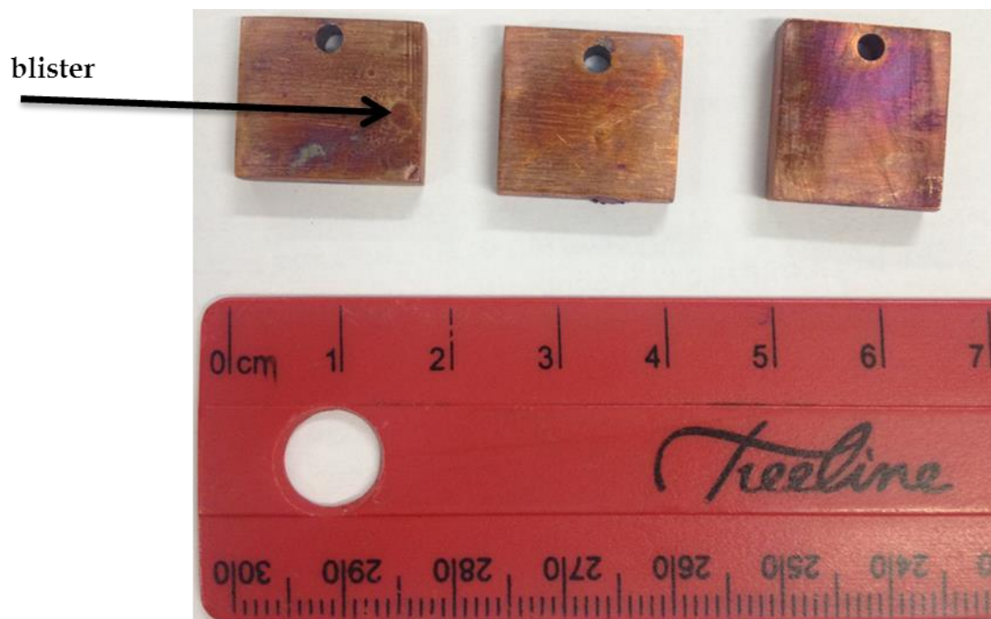
Figure 4.17: Heat-quenched of the copper electroplated samples.
