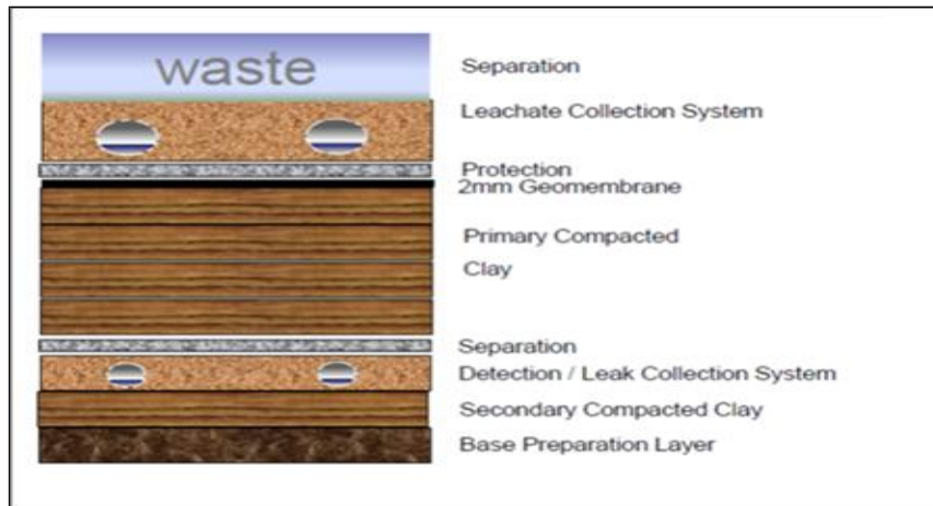
Figure 2-26: The different lining layers of the construction of the new Eskom coal stock yards (Savannah Environmental (Pty) Ltd et al., 2012)
