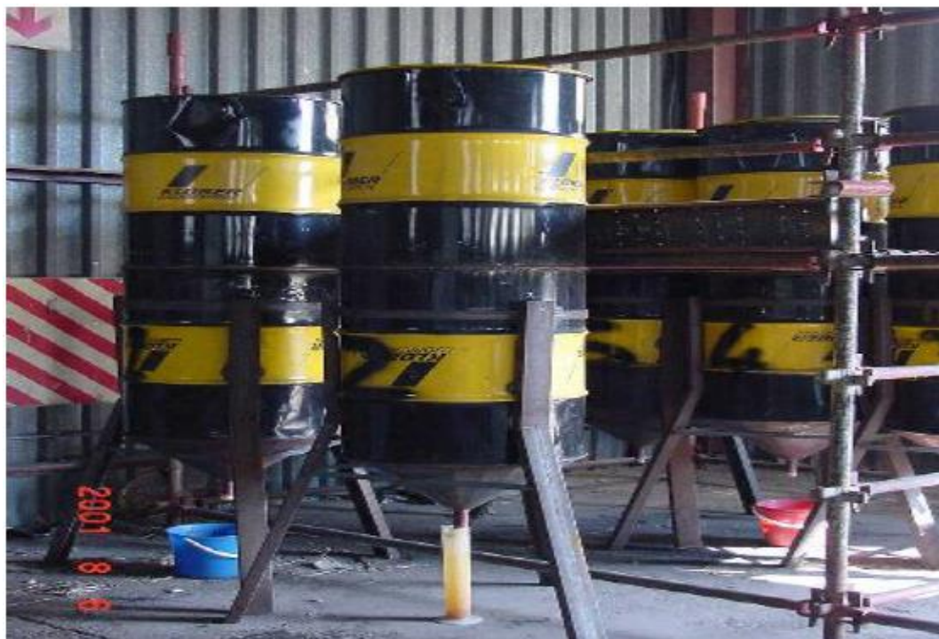
Figure 2-14: Drainage drums used by Cumming (2003)
