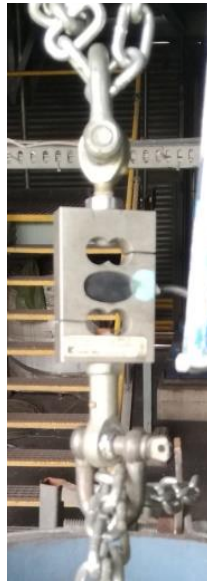
Figure 3-7: Load Cell with shackles
