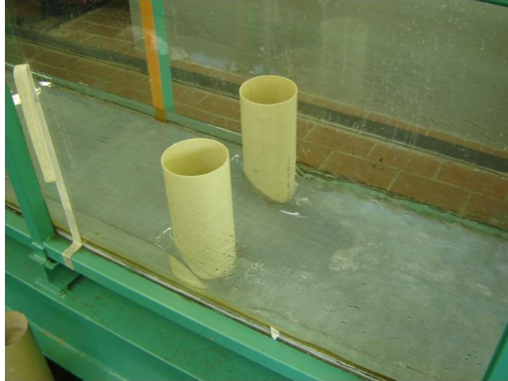
Figure 2: 2 cylinders (diameter = 0.11m) showing varying flow depth around them in flume B
