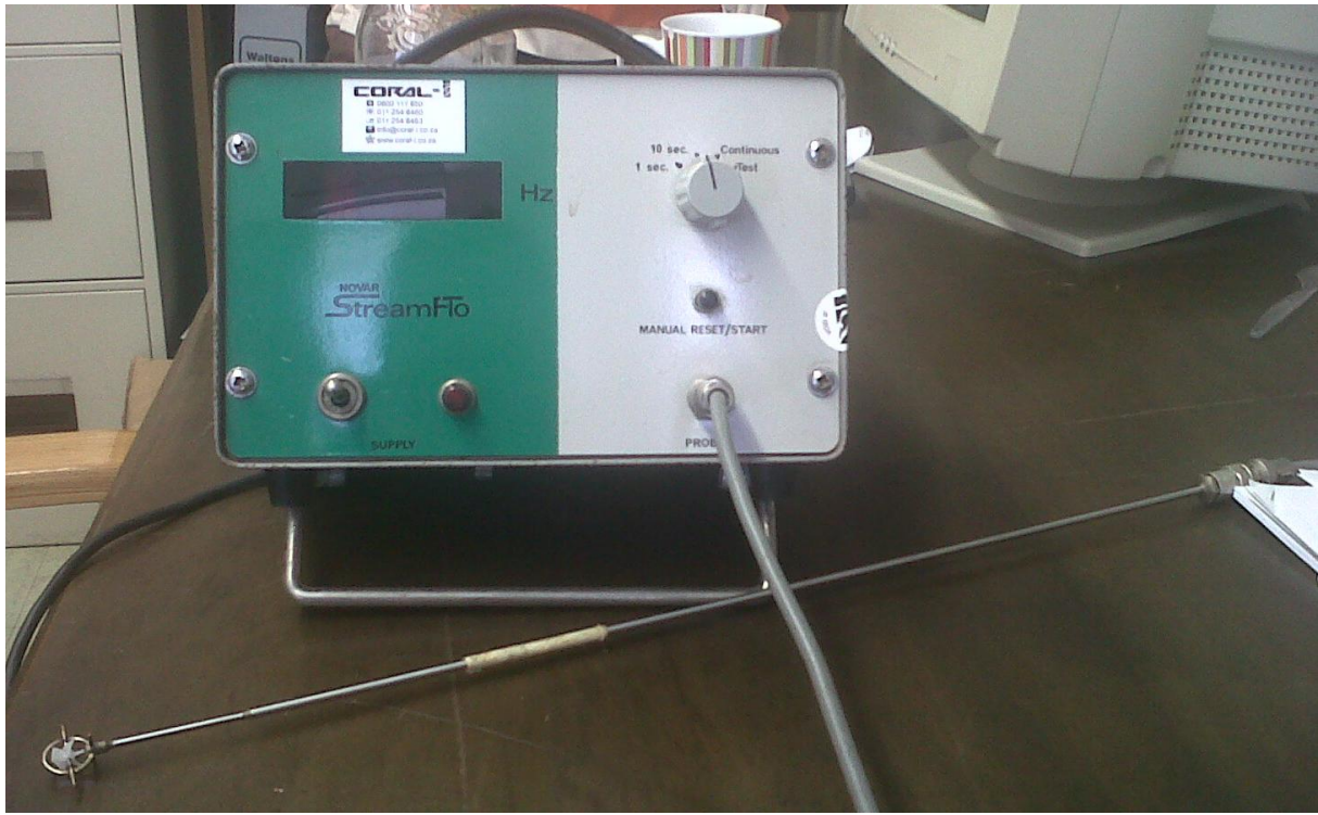
Figure 1: Velocimeter probe with StreamFlo current amplifier that displays readings from the velocimeter in Hertz
