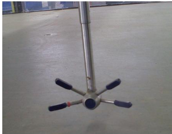
Figure 10: Head of the 3D ADV showing the arms that send and receive the frequency signals
