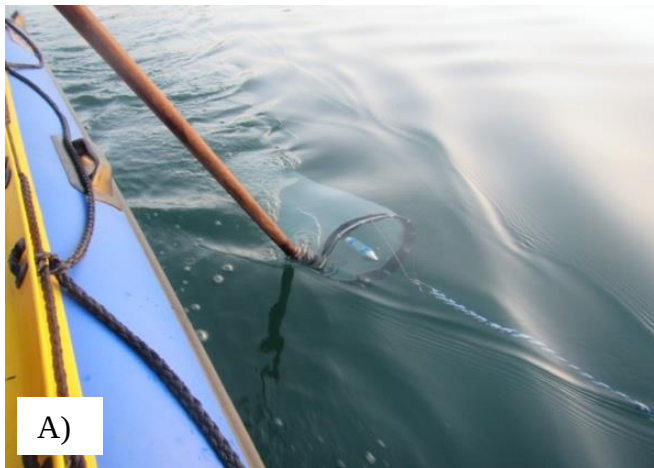
Figure 4. Sampling at Durban Bay A) Deployment of the plankton net used for microplastic surface-water sampling in Durban Bay. B) Photograph of sampling site 7 nearby to a cruise passenger terminal within Durban Bay.
