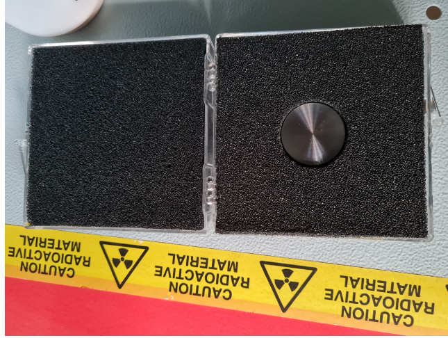
Figure 3.13: The standard radionuclide source prepared by electrodeposition onto a stainless steel disk
