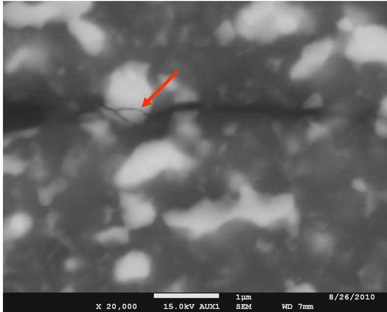
Figure 5-6: Crack branching in the \text{B}_6\text{O}-\text{Al}_2\text{O}_3-\text{Y}_2\text{O}_3-\text{TiB}_2 sample.
