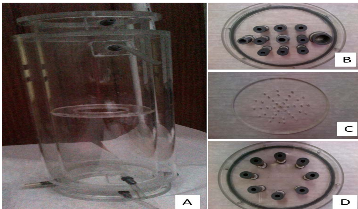
Figure 2.3: A picture illustrating the four main components of the MFC reactor (A). The main cylinder (B) the top lid, (C) perforated plate and (D) the bottom lid.
