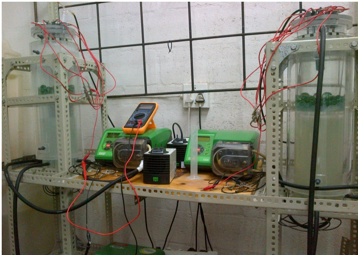
Figure 2.5: A picture of the fully assembled MFC-reactor connected to the pumps (green), O 2 sparger (black and white) and the digital multimeter (orange and grey). The feeding and waste-tank are not shown.
