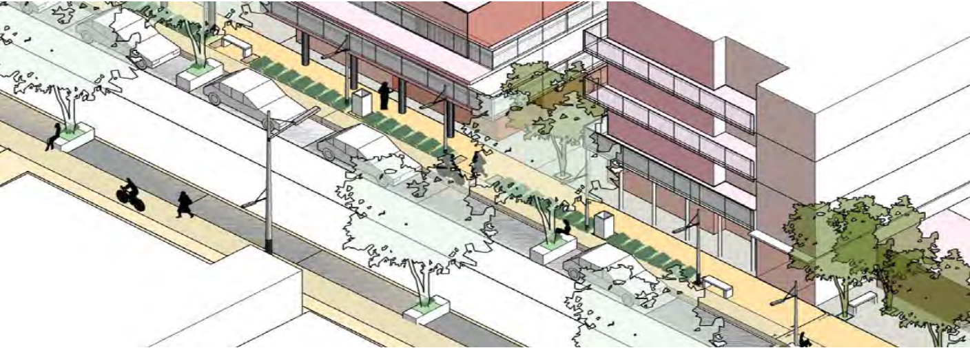
Figure 5.9: Overview of sidewalk detailing in Fourth Avenue indicating on street parking, planters and active ground floor treatment
