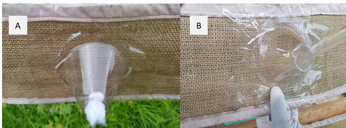
Figure 7: Picture showing WHO cone attached to eave ribbon with a cotton wool plugged on the aspiration hole to prevent mosquitoes from escaping “A” and “B” showing aspiration of mosquitoes in the cone using mouth aspirator.
