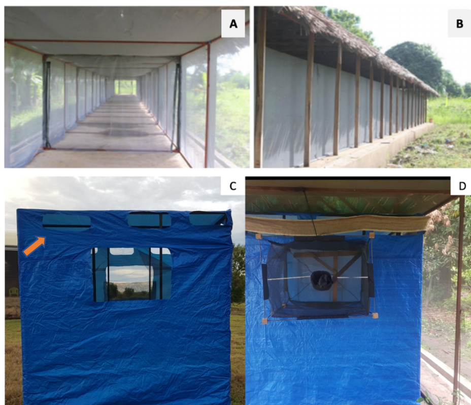
Figure 6: The large tunnel-shaped semi-field cage, within which the study was conducted, and the experimental huts used ( A: Inside view; B: outside view; C: experimental hut with open eaves represented by the orange arrow, without exit trap or eave ribbon; D: hut with fitted ribbon and window exit trap). Source (Mmbando et al. , 2015)
