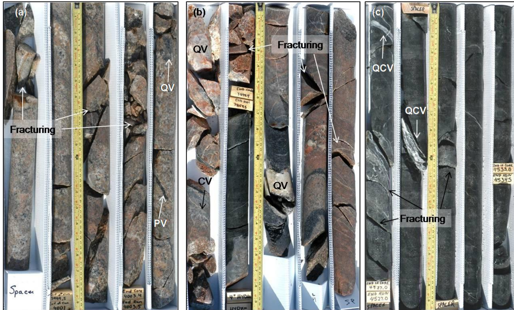
Figure 2.21: Corebox photographs showing fracturing within containing varying amounts of Cal, Py and Qz within the (a) massive megablock granite (Corebox 165), (b) the biotite schist xenoliths in the upper granite megablock (Corebox 147) and (c) the upper amphibolite megablock (Corebox 224). Abbr.: Cal = calcite; CV = calcite vein; PV = pyrite vein; Py = pyrite; QCV = quartz and calcite vein; Qz = quartz.
