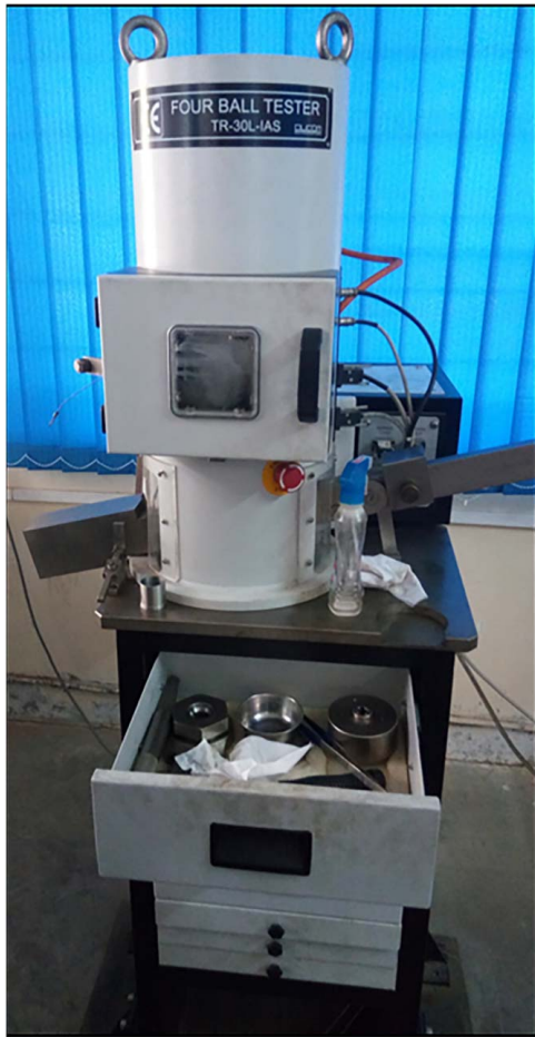
Fig. 4 Illustration of the four-ball tribometer test setup
