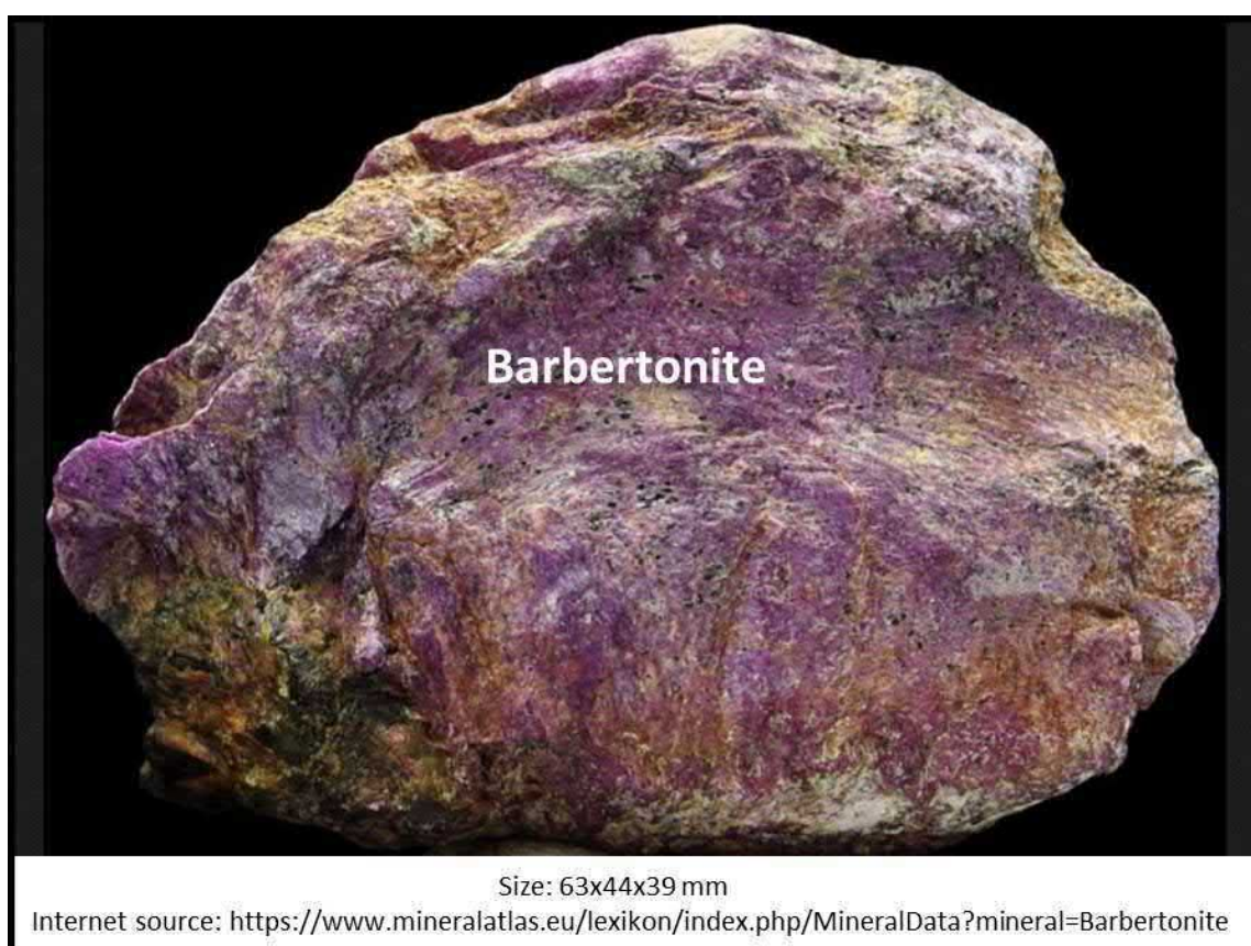
Figure 2.2 Hand specimen of barbertonite (stichtite-2H), a lilac-to-purple chromium hydrotalcite mineral. It is a polytype of, and usually co-occurs with Stichtite-3R (Mills et al. , 2011).
