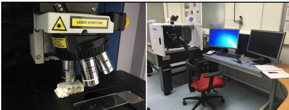
Figure 6. Analytical and data-processing instruments. (A) Sample MJS mounted on a stage prior to analysis. (B): Hardware coupled with spectrometer for data acquisition, processing, and export.
