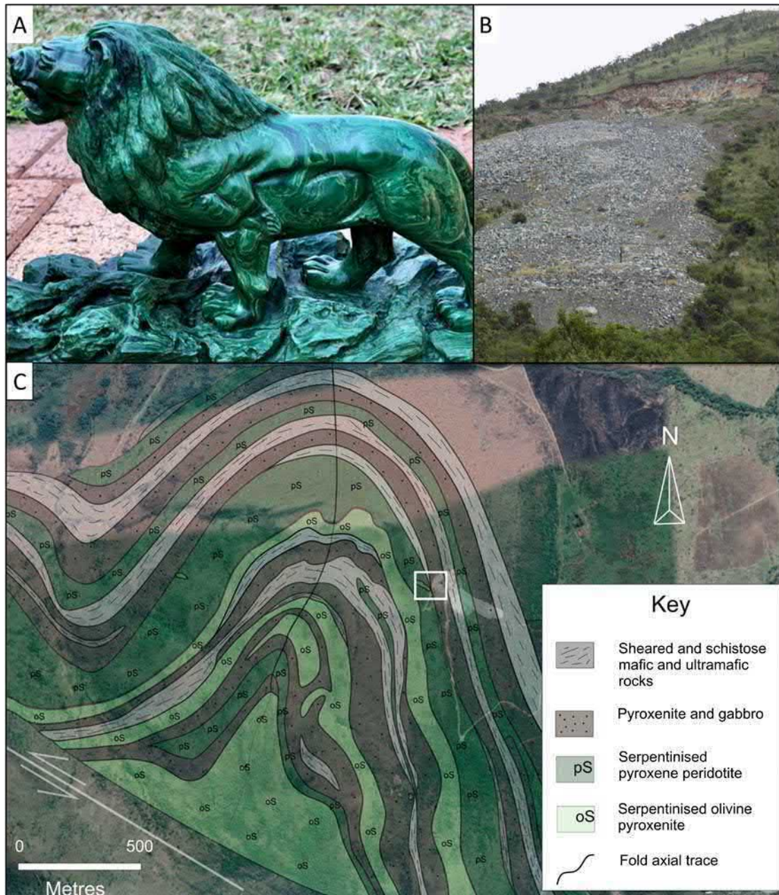
Figure 2.5 Background of the old Handsup Mine. (A) Polished verdite ornament sourced from the quarry. (B) View of the unrehabilitated verdite quarry visible from the R38 road situated within the Jamestown Schist Belt. (C) Modified geological map of the Handsup Layered Ultramafic Complex (Anhaeusser, 1975) superimposed on a Google Earth image. White rectangle mark shows that the Handsup verdite quarry is situated at a lithological boundary between a pyroxenitic serpentinite and a metagabbro associated with a pyroxenite.
