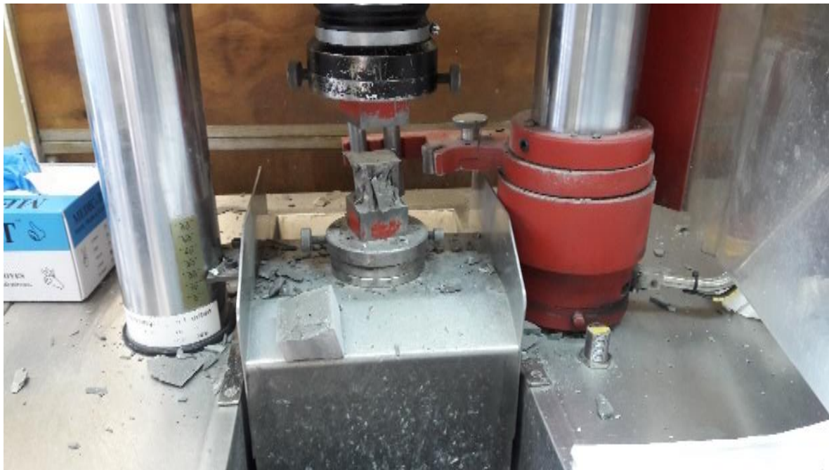
Figure 0.19 The compressive strength testing process
