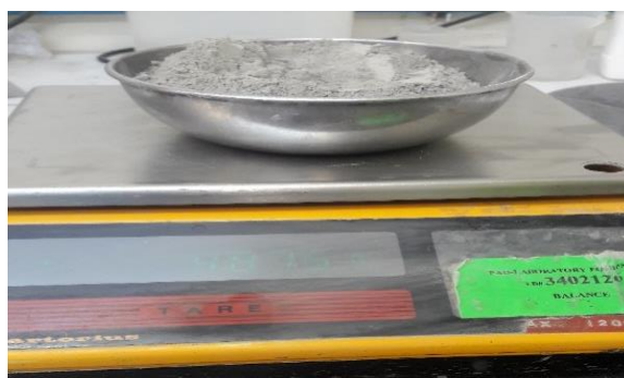
Figure 0.2 Weighing of cement
