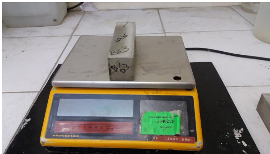
Figure 0.16 Slurry prism weighing process
