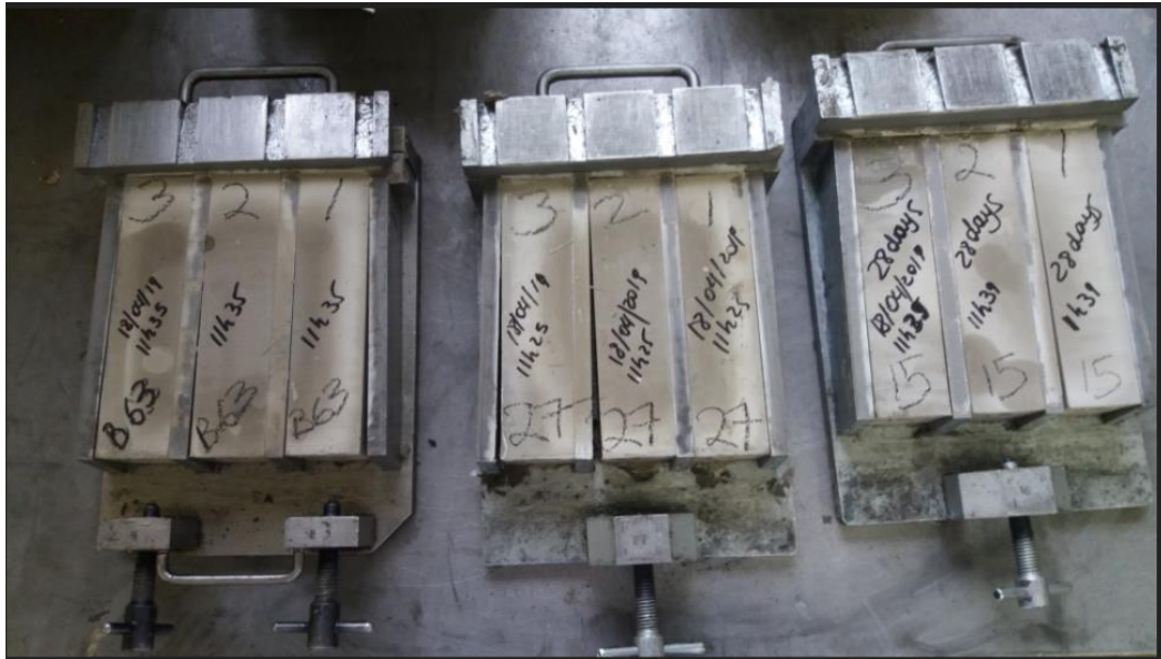
Figure 0.15 Sample demolding process
