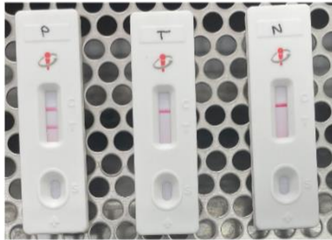
Figure S1 Cell cultures were free from mycoplasma contamination. To ensure cell cultures were free from mycoplasma contamination, the MycoStrip® mycoplasma detection kit (Invivogen) was used according to the manufacturer's instructions. P = positive control, T = THP-1 sample, N = negative control.
