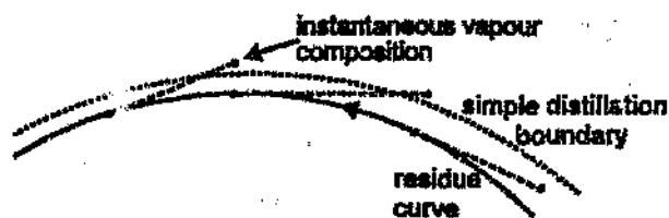
Fig. 2.3 The vapour product from a residue curve may lie on the other side of a simple distillation boundary.
