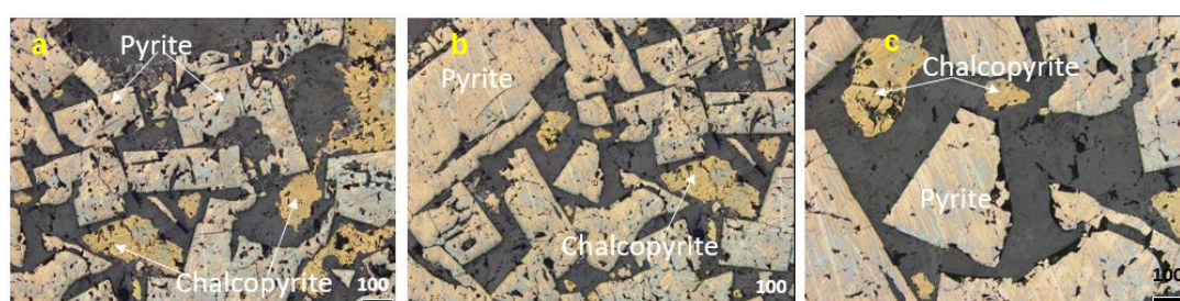
Figure 6-9. Cubic pyrite within siltstone and carbonate layers of Sequence 6, Shantumbu. Chalcopyrite (Ccp) is sub-hedral to anhedral (a to c). All images in plane polarised reflected light. (a) Sample E2215B
