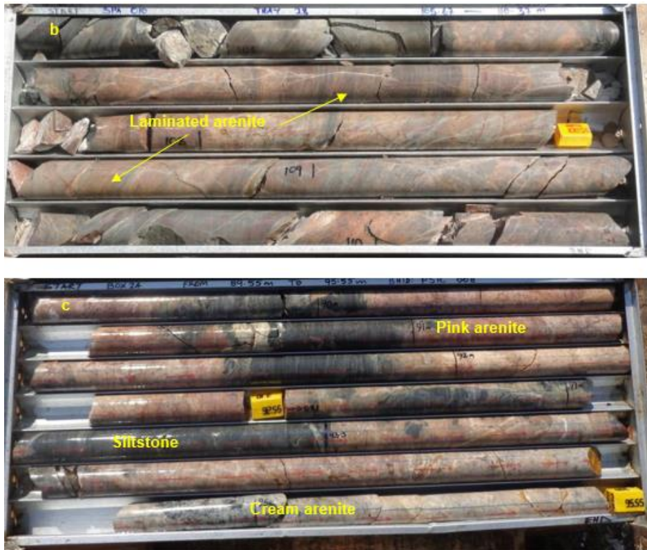
Figure 4-6. Lithologies of Sequence 2, Shantumbu. (a) Sequence 2 shows rounded to sub-rounded dark grey plagioclase-quartz patches in SPA005 (at a depth from 132.35 to 136.65m). (b) Laminated arenite (SPA018 at a depth from 105.67 to 110.37m). (c) Interbedded arenite and siltstone layers (PSH008; at a depth from 89.55 to 95.55m).
