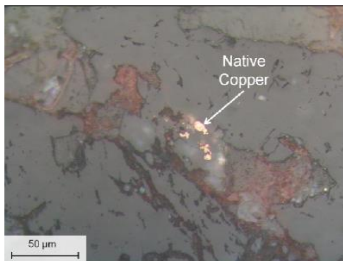
Figure 6-4. Native copper within the calc-silicates of the marine transgression zone from sample H08304 from PSH008 at a depth of 109.20m, Sequence 3/4, Shantumbu. Image in plane polarised reflected light.
