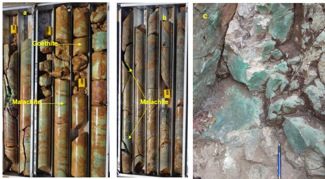
Figure 4-4. Fine-grained arenite of Sequence 1, Shantumbu. (a) Fine-grained arkose of Sequence 1 hosting malachite and chlorite (PSH008). (b) Malachite along bedding and fracture planes, hosted by fine-grained grey arkose of Sequence 1 (PSH008). (c) Outcrop of fine-grained arkose hosting malachite mineralisation at Copper Hill, Shantumbu.
