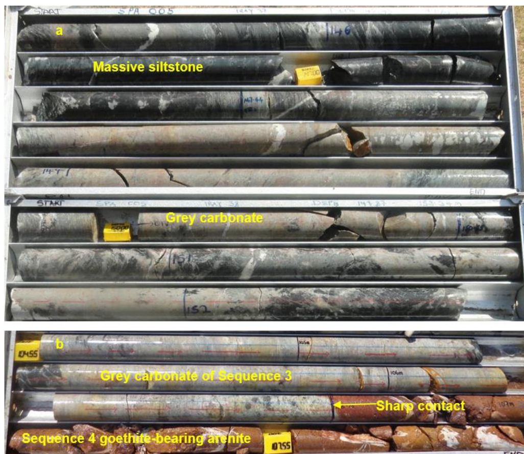
Figure 4-8. The sub-aqueous siltstone and carbonate lithologies of Sequence 3, Shantumbu. (a) Siltstone and grey carbonate of Sequence 3 in SPA005 (145 – 153m) overlain by grey carbonate and massive siltstone layers of Sequence 3 (PSH008 at a depth of 104 to 108m). (b) The goethite-rich arenite of Sequence 4 caps the grey carbonate of Sequence 3.
