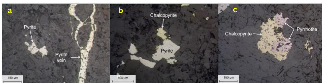
Figure 6-7. Sulphides within Sequence 5, facies b, Shantumbu. (a) Post-brecciation veins composed of anhedral pyrite, pyrrhotite and chalcopyrite (H08292 from PSH008 at a depth of 52m). Sulphide grains (H08292 from PSH008 at a depth of 52m) both within veins and the matrix of the breccia, as shown in (b) and (c) (H08295 from PSH007 at a depth of 136.47m). All illustrations are in plane polarised reflected light.
