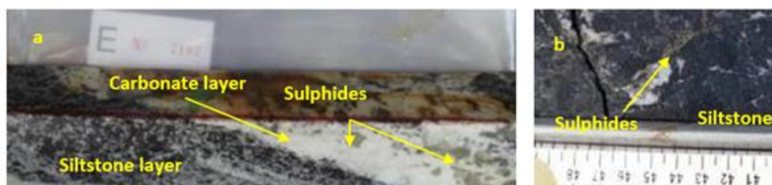
Figure 6-8. Sulphides are hosted by both siltstone and carbonate layers in Sequence 6, Shantumbu; quarter core sample. (a) Large anhedral sulphides grains within carbonate (E2192 from SPA014). (b) Fine-grained sulphide within siltstone; core sample.
