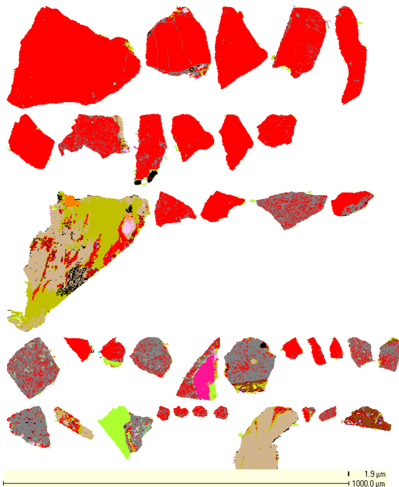
HILG 21. Uraninite is the dominant uranium bearing phase, the map shows a bimodal grainsize distribution, with finer grains predominantly uranium oxide-silicates, a product of surface weathering. The chlorite is a possible result of the weathering of biotite, where uraninite is found II to the cleavage. Uraninite in this sample is up to 300 μ across.
