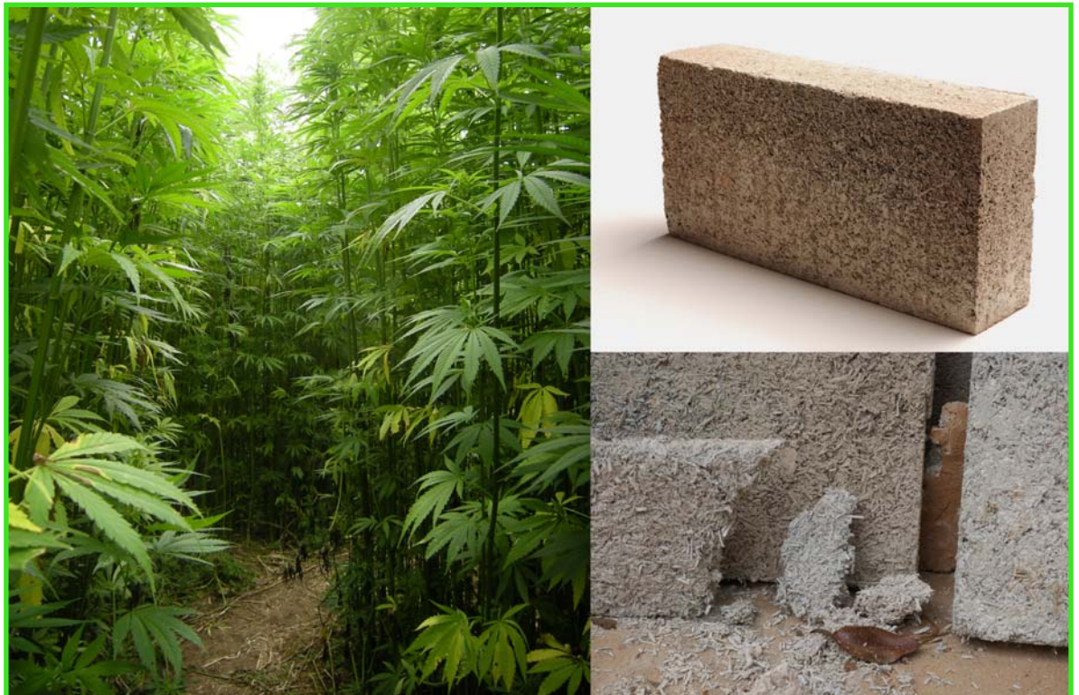
Fig. 5.33: Hemp plant and Hempcrete blocks. This is an environmentally friendly building material and is also incredibly strong. (Source: De Smit, 2010, and Geiger, 2011)
