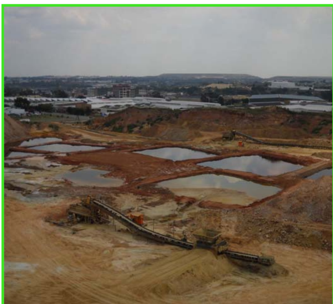
Fig. 5.4: Mine tailings in Johannesburg with acid mine drainage. (Source: author, 2011)
