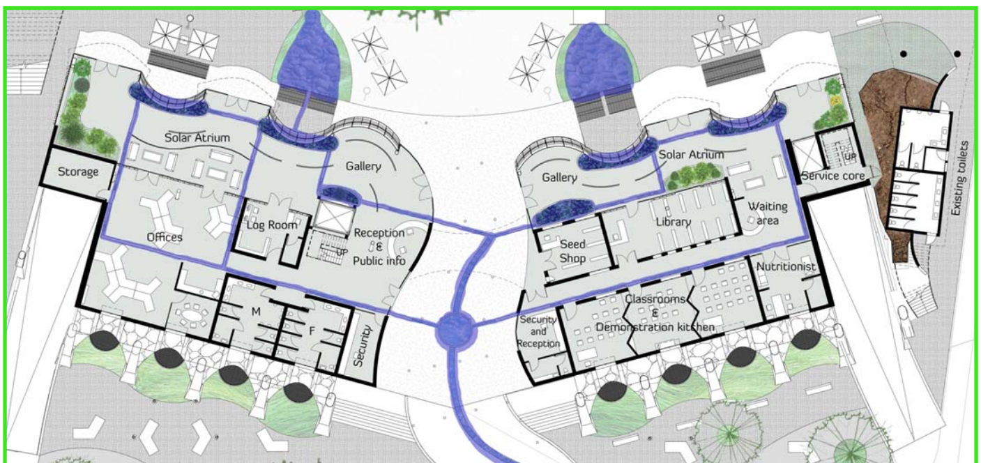
Fig. 5.32: The water channel in the ground floor of the design.
