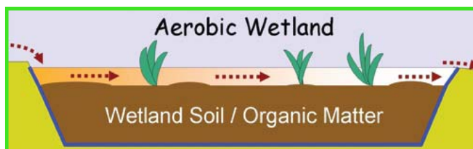
Fig. 5.5: Aerobic wetlands soil treatment. (Source: Zipper et al., 2011: 3)
