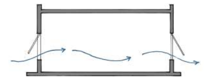
Figure 3.12: Section showing Cross-ventilation (Author, 2023)
