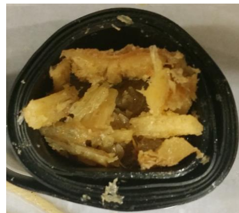
Figure 3.2.7: Photograph of the tape enveloped specimen post current treatment
