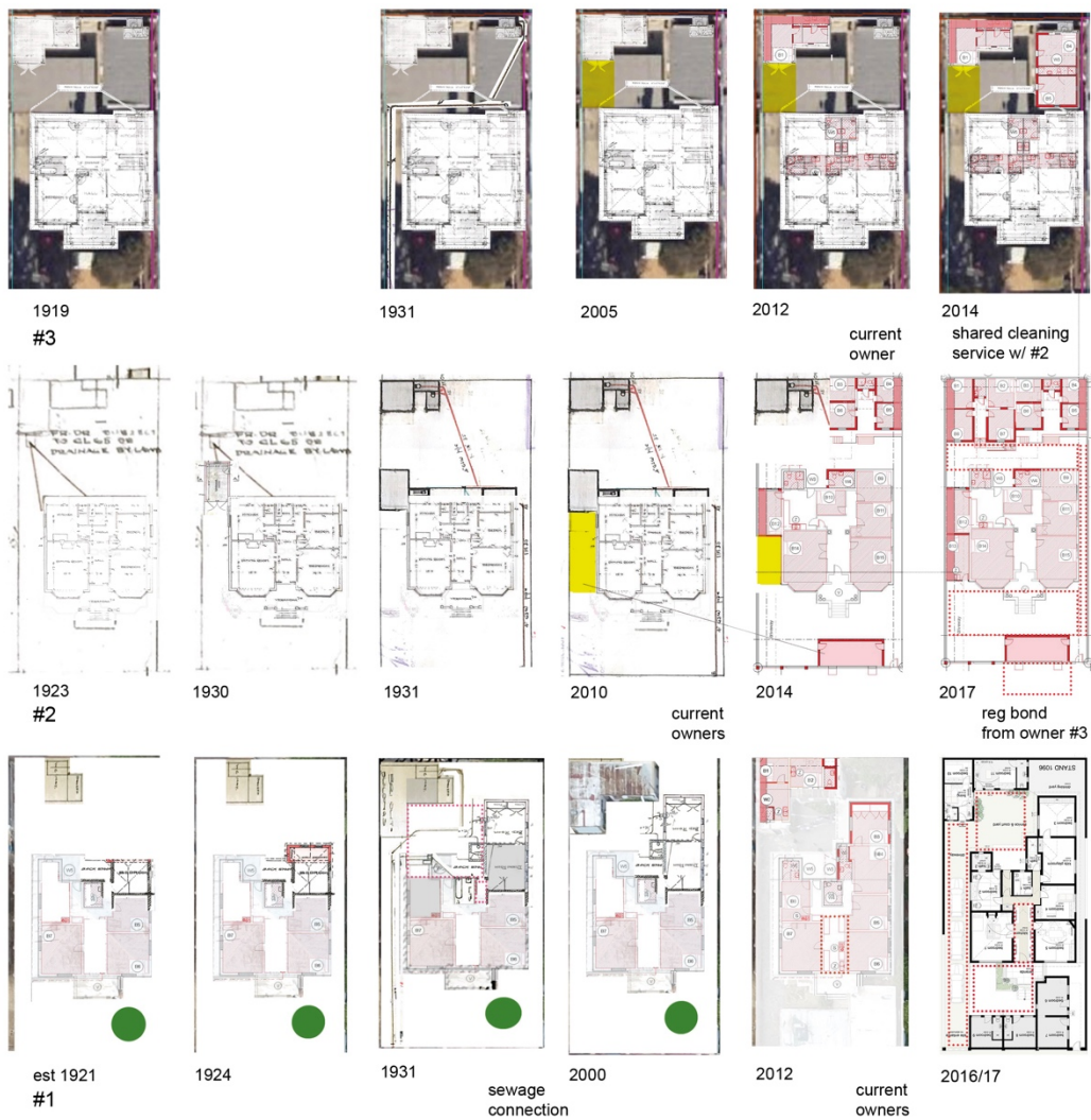
Figure 17: Case Studies #1, #2, #3, change over time; Storyboard of physical alteration, reconstruction of “as built” (author’s own, 2023)
