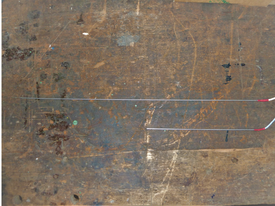
FIGURE A.8: Two PT-100 temperature sensors used in the experiments.
