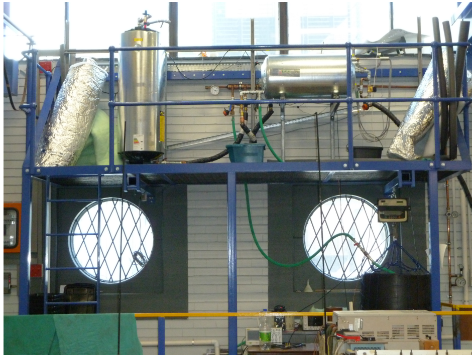
FIGURE A.1: Test bed for water heater testing.
