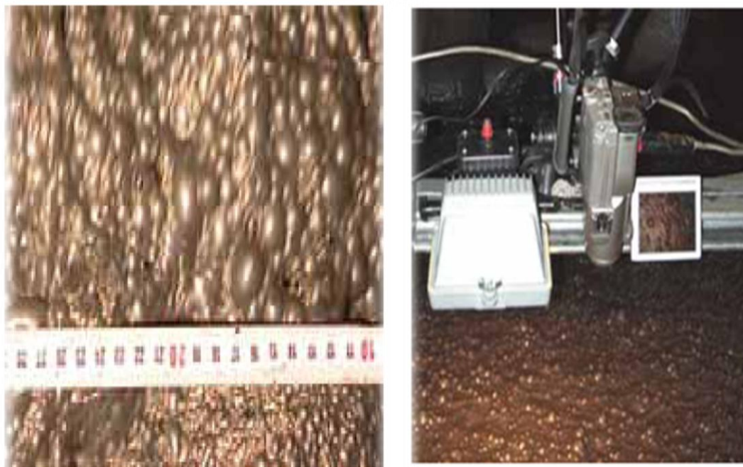
Figure 2.5: SmartFroth camera installations for froth surface bubble size (Forbes, G., 2007)
