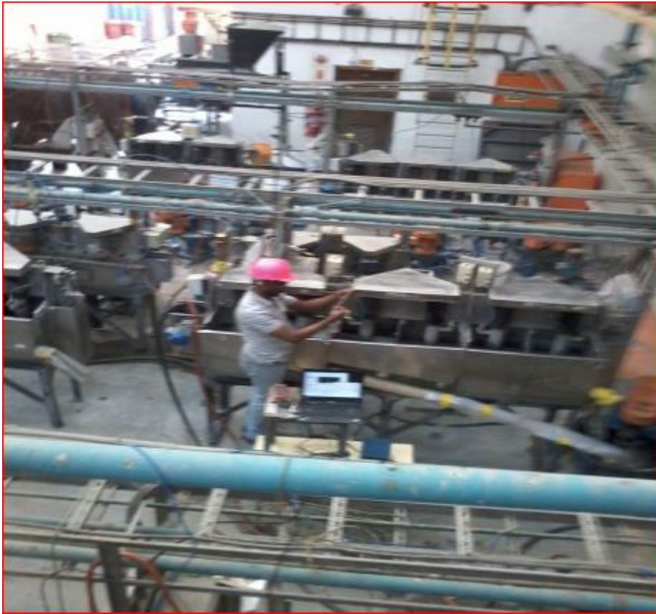
Figure 3.3: Mintek pilot plant, showing secondary rougher bank which consists of 6 cells and installation of probe for froth bubble measurement.
