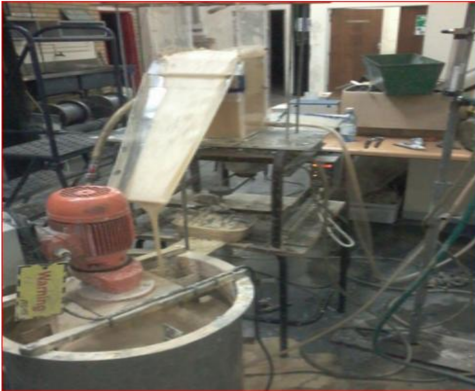
Figure 3.2: Picture of the pseudo-steady state flotation experimental equipment in the Mineral Processing laboratory at University of the Witwatersrand.
