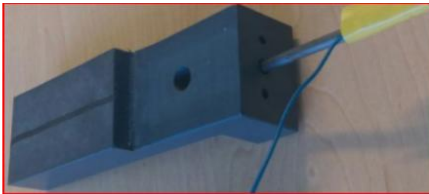
Figure 3.6: Picture of probe release, showing probe and pin holes.
