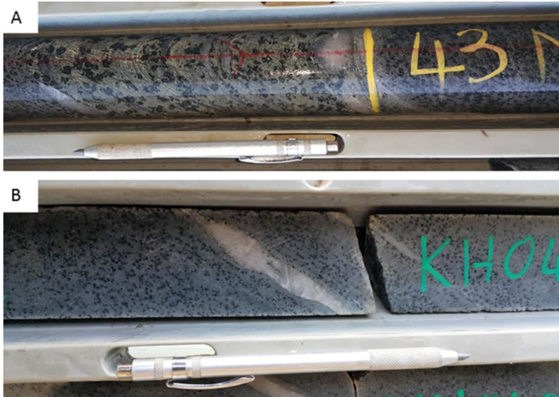
Figure 4.2: Core photographs showing the speckled schist (biotite chlorite schist) from KM12-01 at depth 42.8 m-43.8m. A) Typical local shearing associated with biotite-chlorite and sericite alteration. B) Speckled nature of the biotite chlorite schist with a boudinaged quartz vein.
