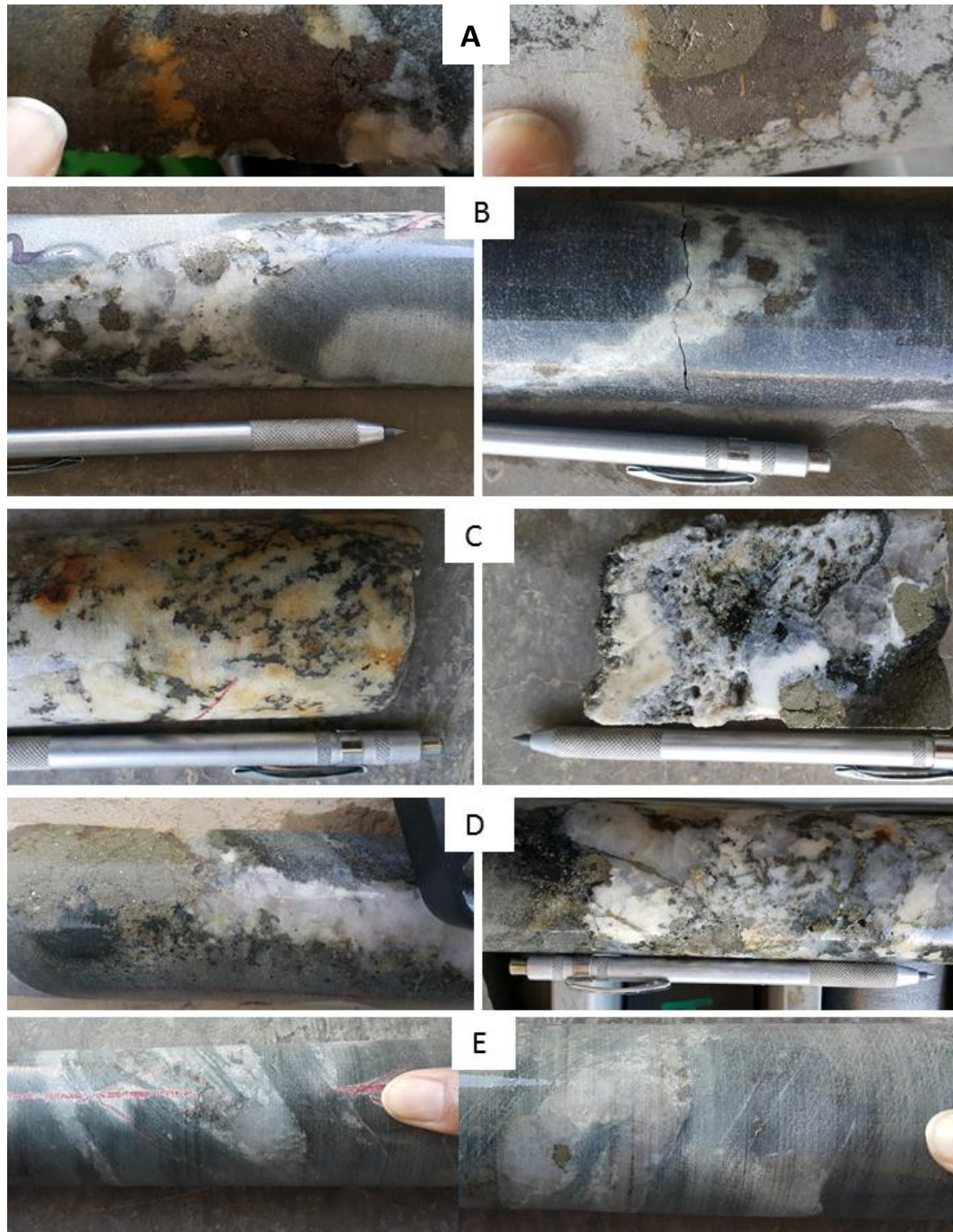
Figure 4.9: Core photographs showing quartz-carbonate veins and the sulphides hosted within them. A) Patches of pyrrhotite, chalcopyrite and pyrite within a quartz-carbonate vein. Pyrite and chalcopyrite form rims within the chalcopyrite grain (KM12-01). B) Patches of pyrrhotite and chalcopyrite within a quartz-carbonate vein (KM12-01). C) Disseminated pyrrhotite and pyrite patches in a carbonate dominated vein (KM12-01 at 112.6 m-113 m). D) Patches of pyrrhotite, pyrite and minor chalcopyrite within quartz-carbonate veins and within fractures between veins. E) Folded quartz veins within a chlorite sericite schist with minor patches/blebs of pyrrhotite and chalcopyrite (KM12-02 at 238.8 m).
