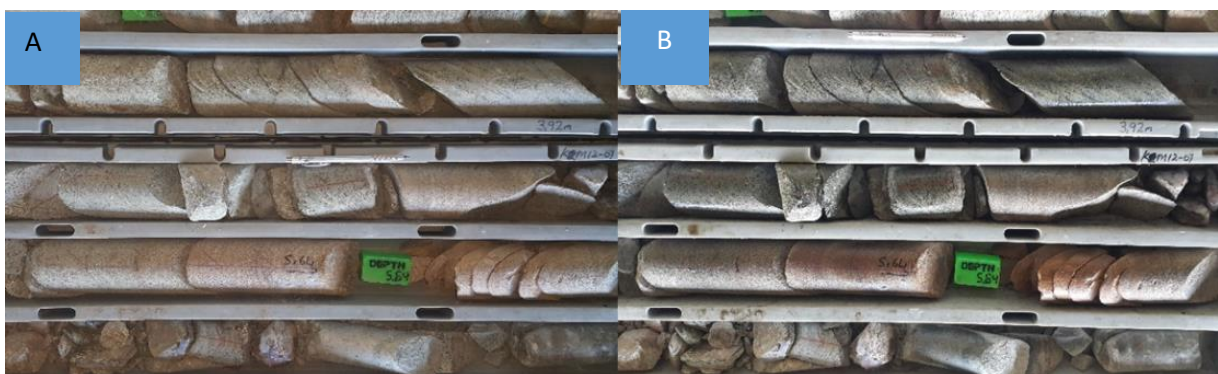
Figure 4.1: Core photographs of the dry (A) and wet (B) highly fractured and foliated muscovite schist from the Kariam Prospect, borehole KM12-01 around 5.64m.
