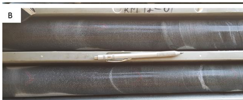
Figure 4.4: Core photographs of the biotite schist, from KM12-01 at 115.1 m-116 m. It is a massive unit with little or no foliation, rarely veined and contains no sulphides.
