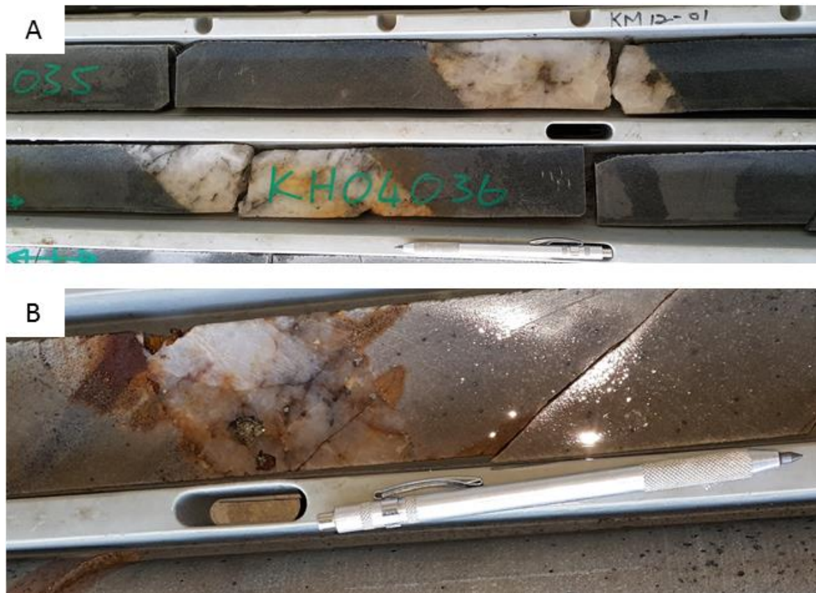
Figure 4.5: Core photographs of the quartzitic schist. A) Quartz-carbonate veins cross cut the foliation of a medium grey quartzitic schist, KM12-01 at 110 m -111 m. B) Cream bleached schist which contains cross-cutting chalcopyrite and pyrite-rich quartz-carbonate vein and disseminated magnetite within the matrix, from KM12-01 at 397.3 m.
