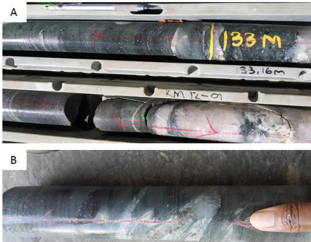
Figure 4.3: Representative core photographs of the chlorite sericite schist. A) From borehole KM12-01 at 133- 134 m, it shows a green-grey schist with quartz veins parallel to foliation in range of >1 mm to 30 cm wide. B) Chlorite sericite schist with folded mineralised (chalcopyrite and pyrrhotite) quartz veins developed within the foliation (KM12-02 at 238.3 m).
