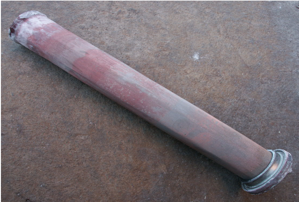
Fig 7.7: Corrosion clearly visible on Monel filter
