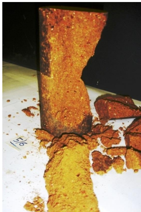
Figure A.10 Compounded specimen 2619-UCM-G5/6 after testing and after removal of loose fragments.
