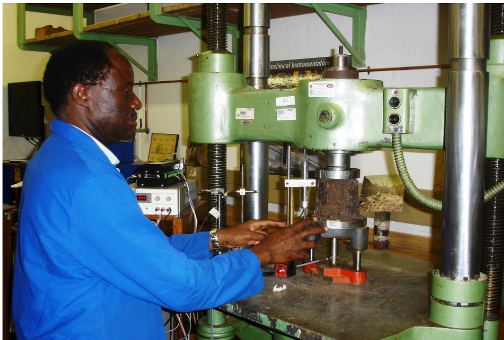
Figure 3.1 Experimental set-up for testing stabilized soil specimens
