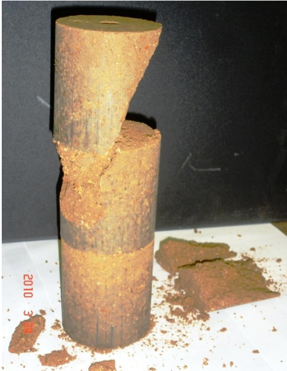
Figure A.11 Compounded specimen 2619-UCM-G7/8/9 after testing and removal of loose fragments.
