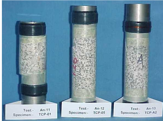
Figure 3.12 Test specimens with different height-to-diameter ratios
