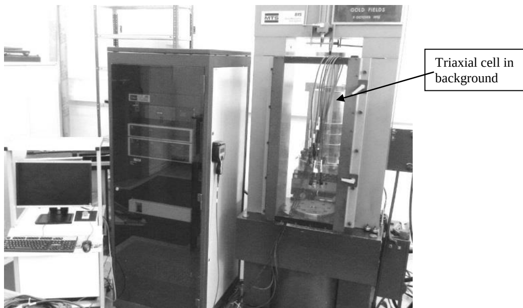
Figure 3.10 The MTS servo-controlled testing machine
