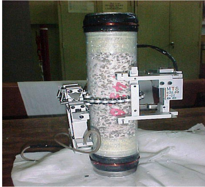
Figure 3.11 The MTS Transducers for axial and circumferential strain determination
