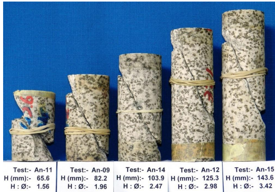
Figure 3.15 Mode of failure of Anorthosite test specimens
