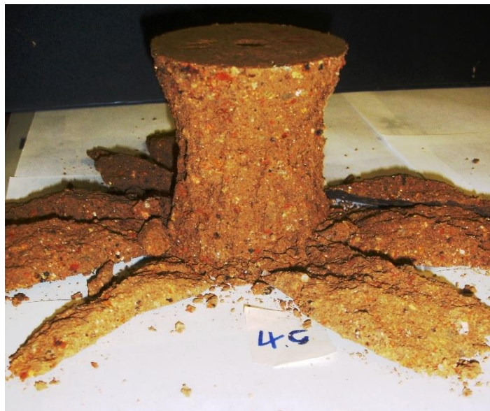
Figure A.8 Test Specimen 2619-UCM-G4 after testing and removal of loose fragments.
