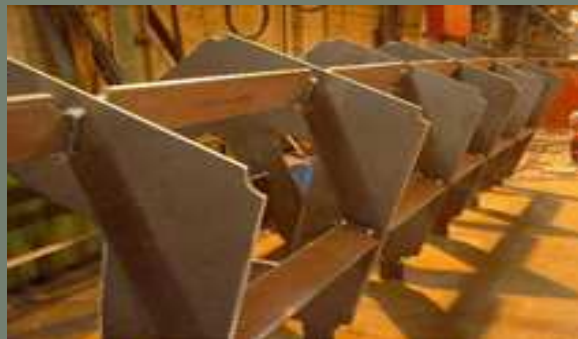
Figure 7.14: Segmented steel plates
