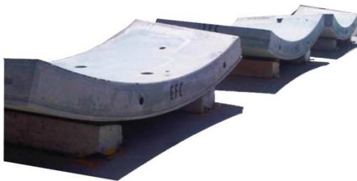
Figure 7.5 : Geopolymer Concrete, https://www.tunneltalk.com/TunnelTECH-Jan2014-Sustainable-Earth-Friendly-Concrete-for-high-durability-tunnels.php
