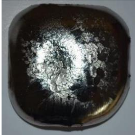
Figure 3-2. As-cast (~50 x ~30mm) Ti-5Cu alloy button (50g).
