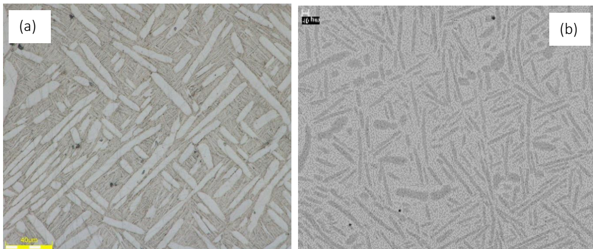
Figure 4-23. Microstructures of as-cast Ti-5Cu: (a) OM image, showing ( \alpha Ti) (light contrast) and \text{Ti}_2\text{Cu} (dark contrast), (b) SEM-BSE image, showing ( \alpha Ti) (dark contrast) and \text{Ti}_2\text{Cu} (light contrast).
