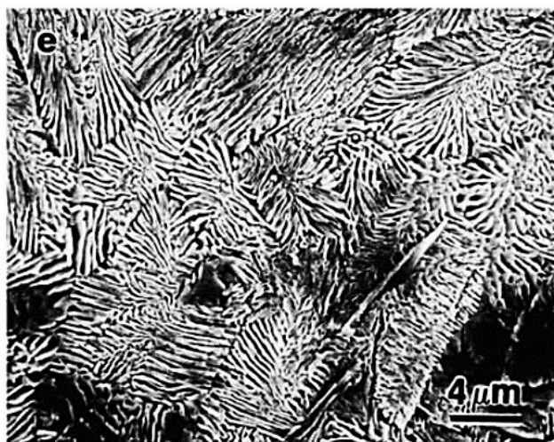
Figure 2-14. Typical microstructure of the as-cast Ti-10Cu (Kikuchi, et al., 2003).
