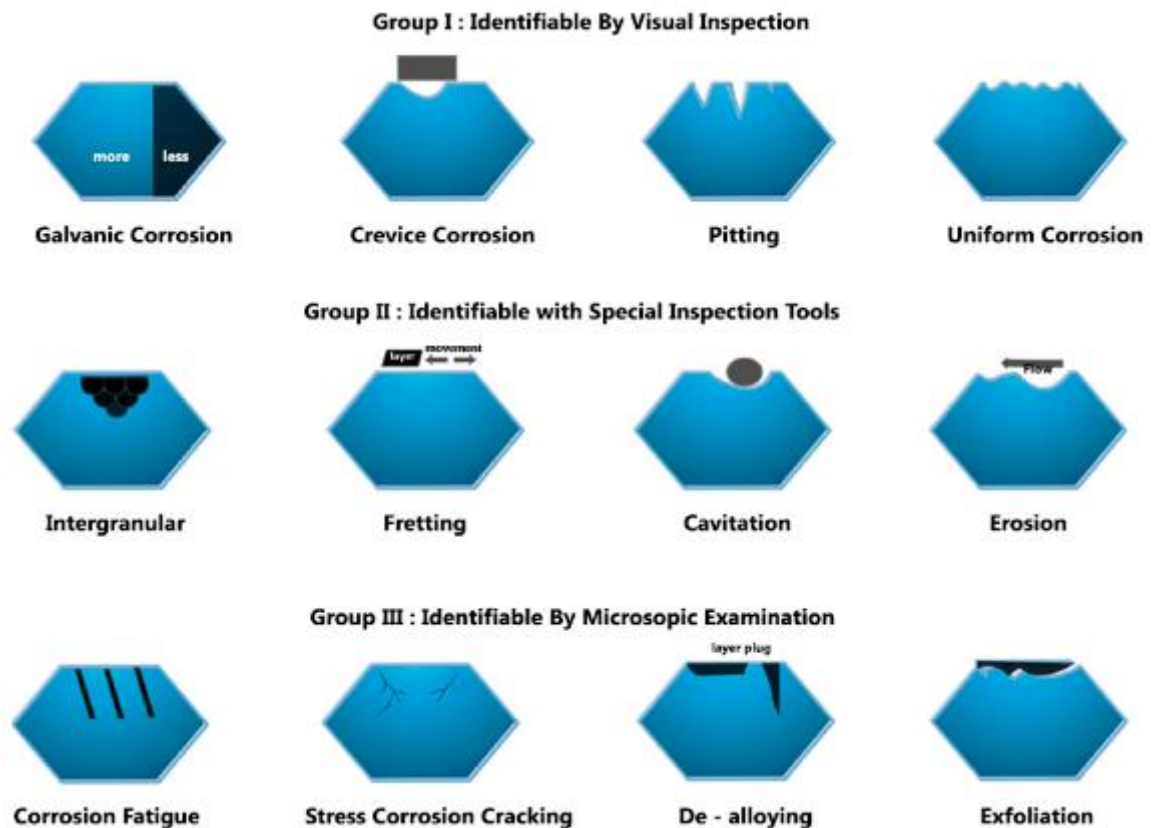
Figure 2-18. Different forms of corrosion (Noumbissi, et al., 2019).
