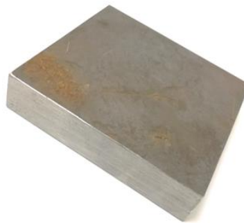
Figure 3.2. Mild steel sample used as substrate.
