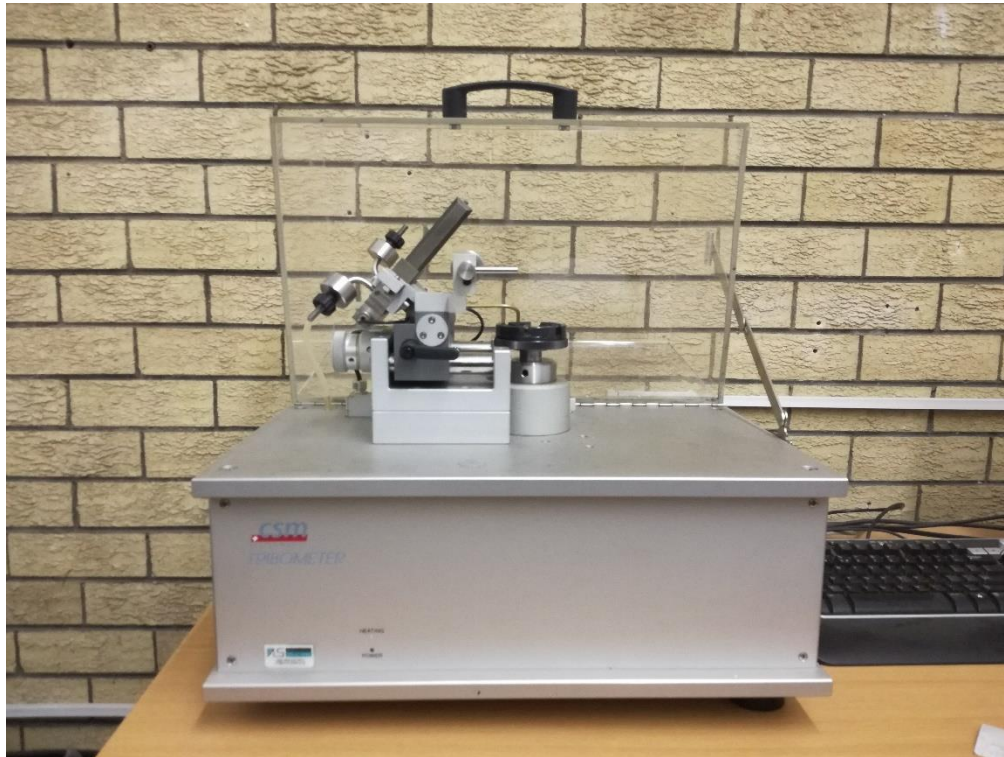
Figure 3.7. CSM Tribometer used for sliding wear testing.
