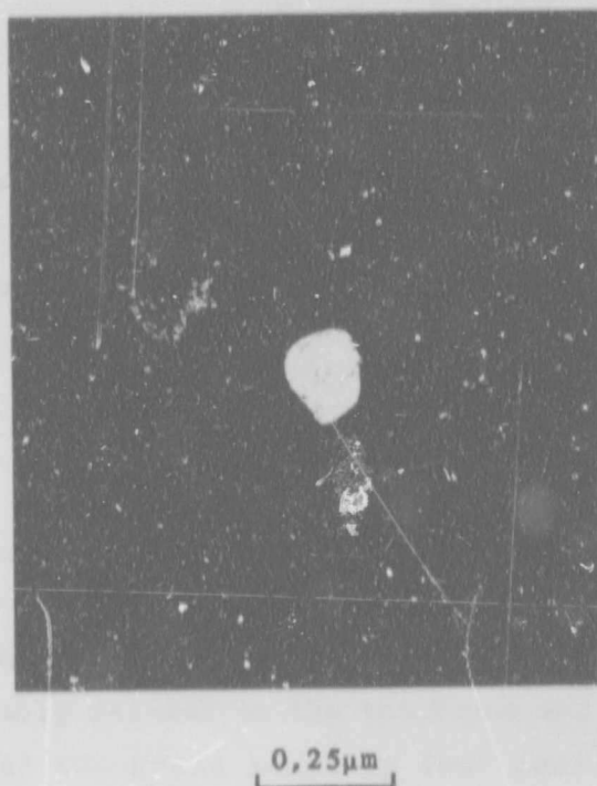
Figure 4.39 Spheroidal precipitate in the V4/0,1 alloy. Note that the grain boundary on either side of the precipitate is 'clean'.
