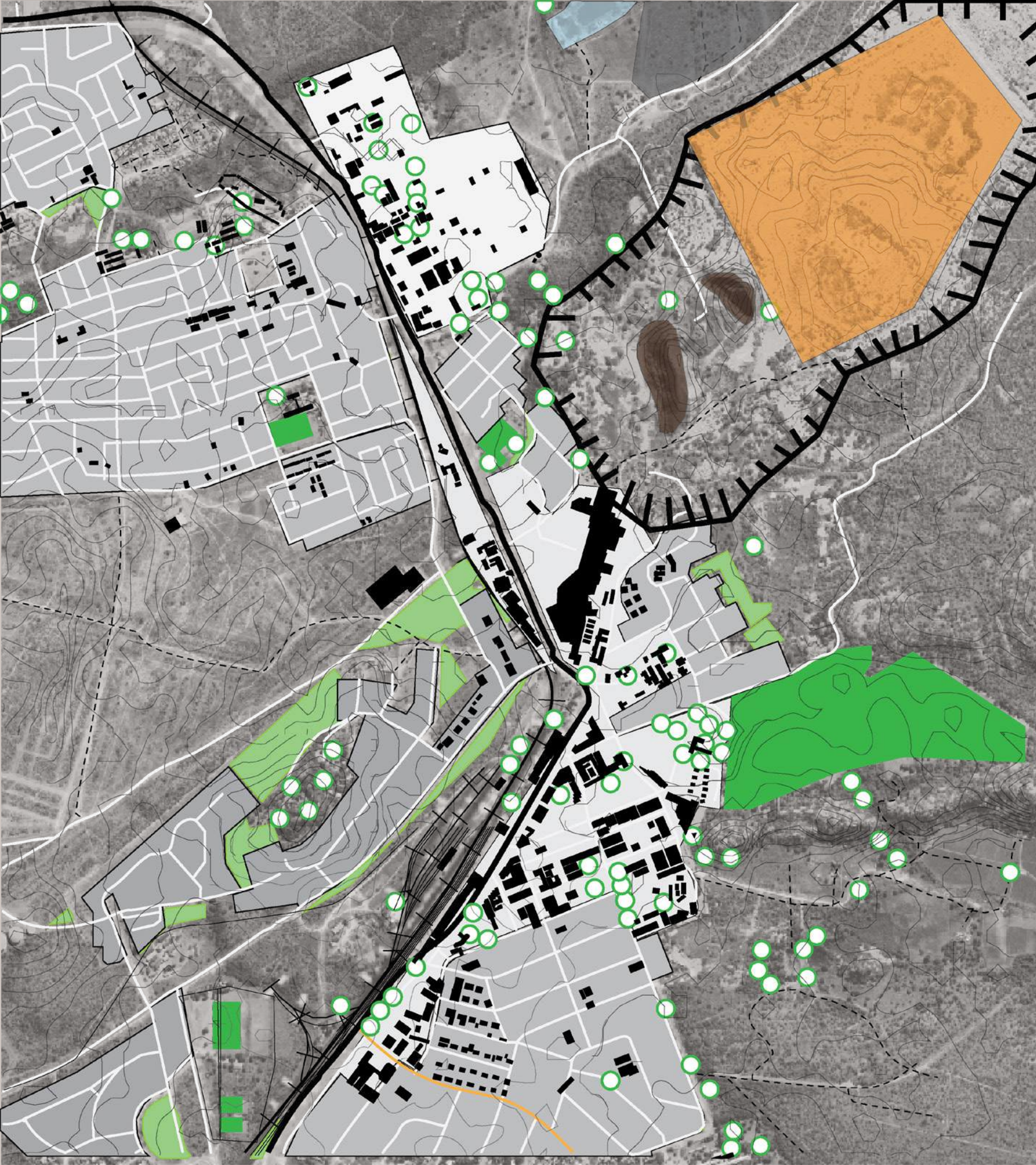
Figure 40: Musina Copper Mine Map in relation to the Land Use Zone. This figure displays a spatial analysis of the Musina Copper Mine concerning the designated land use zones in Musina Town. The map illustrates the mine's position in the Messina Fault Belt, highlighting its proximity to key infrastructure elements such as residential areas, commercial zones, and environmentally delicate regions. It also illustrates how mining activities impact land use, city planning, and environmental conservation efforts. The combination of commercial, residential, industrial, and conservation zoning classifications illuminates the environmental and socioeconomic dynamics affecting Musina's landscape
