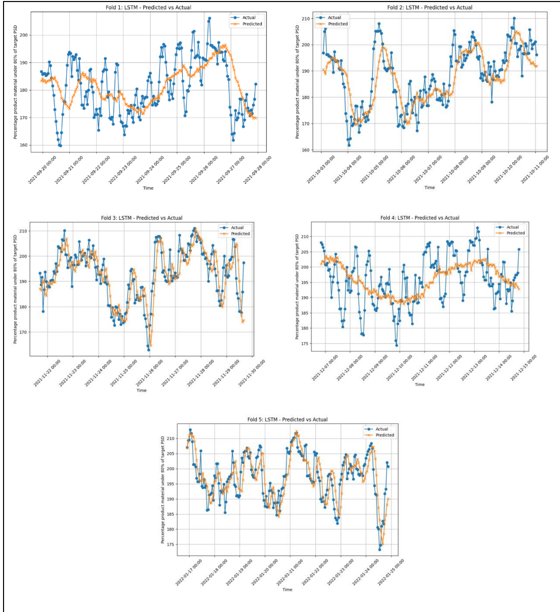
Figure 4.5: The graphs show the predicted vs actual data folds for the percentage product material under 80% particle size distribution (PSD) using the Long Short-Term Memory model
