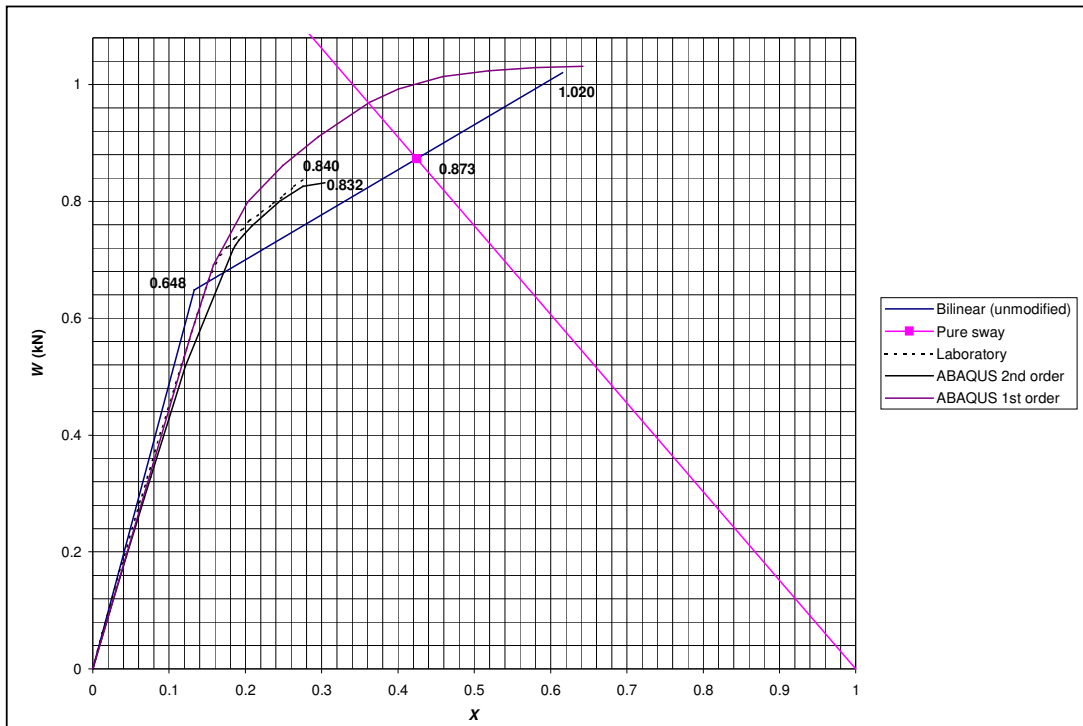
Fig. [4.12] Bilinear W - X graph of 0.33sway frame
