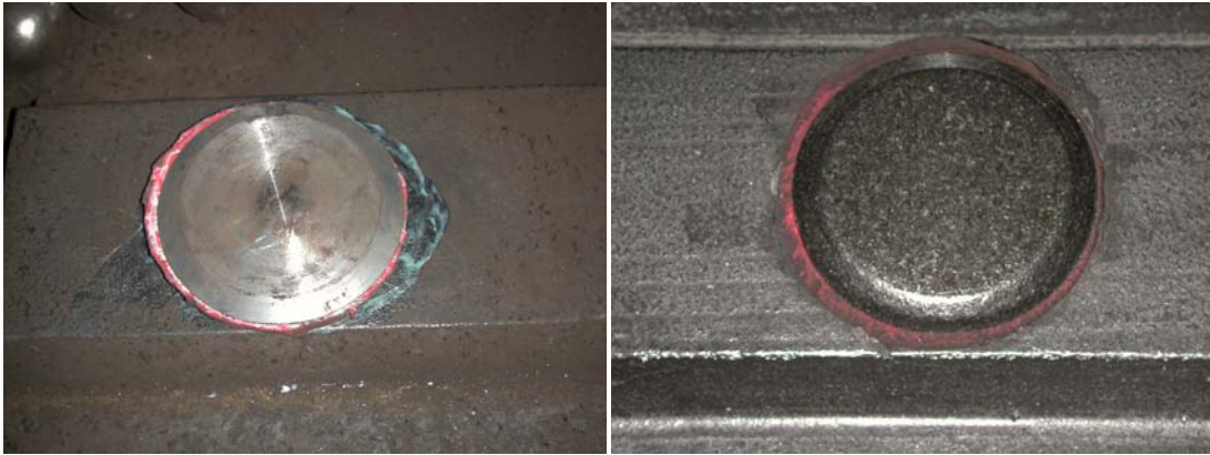
Figure A3.2.3: Pictures of Movement probe M1, taken from inside the mill. Pictures were taken before (left) and after (right) mill testing.
