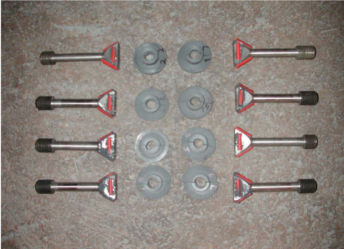
Figure A3.2.1: Conductivity probes (bolts only) including pieces of PVC triangular strips already glued onto the probes. Matching PVC washers included per probe.
