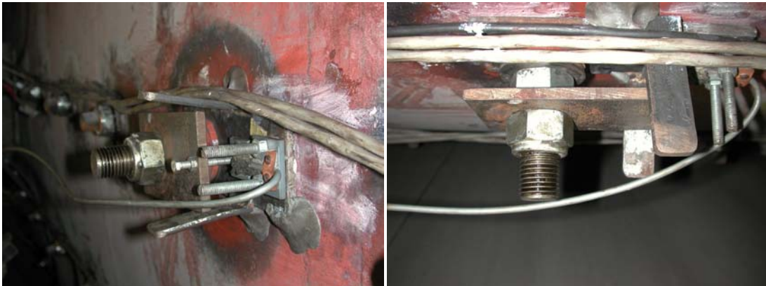
Figure A3.2.4: Movement probe M1 support base and strain gauge.
