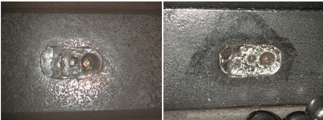
Figure A3.2.5: Laser and photo-detector reflector (PDCR) after installation (left) and after testing (right). PDCR operated for only two tests. Testing of detector after mill tests proved that the detector was faulty, indicating that harsh milling environment affected detector functionality.
