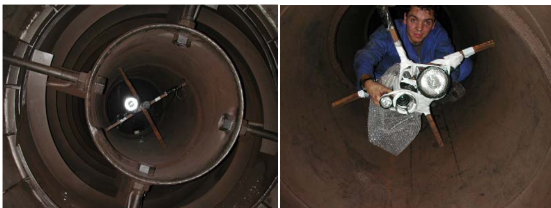
Figure A3.2.7: CCD camera and spot-light (left); Video camera, flashlight and spot-light (right).
