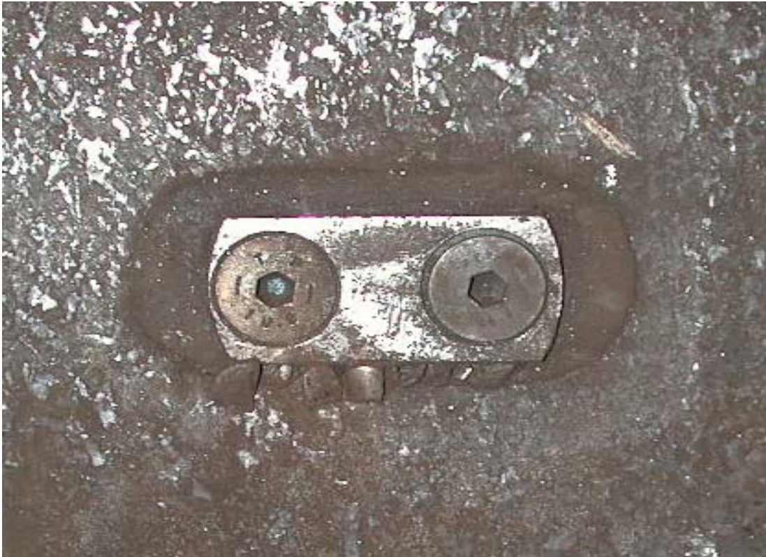
Figure 3.14: Steel particles collecting around conductivity probe (CM1).
