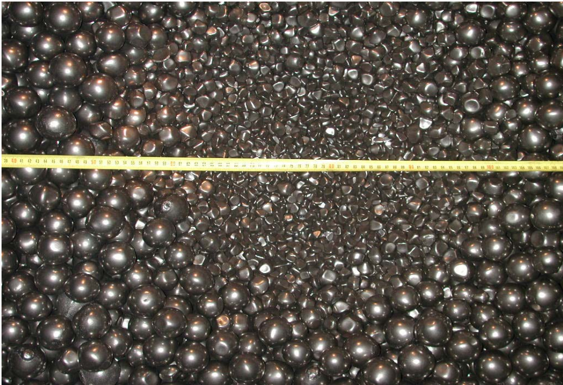
Figure 3.10: Ball load distribution at the surface; 800mm from mill feed drive end in a hole 170mm deep after barring.
