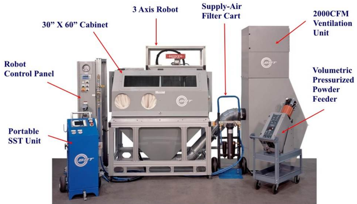
Figure 3.4: Cold spray equipment [ https://www.wits.ac.za/mecheng/research/research-units/cold-spray-research/facilities/ Access date: 5 June 2017].
