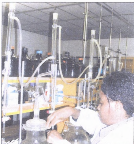
Figure 14. Hydrodistillation of plant material to obtain essential oil.
