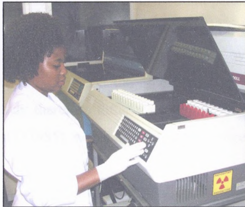
Figure 20. ^{14}\text{C} prostaglandin counted with scintillation counter.
