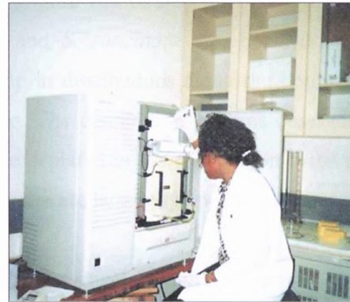
Figure 21. Loading the DNA template onto the gene scanner.
