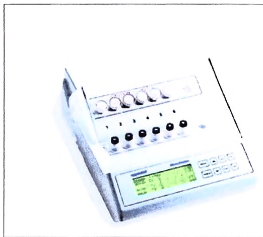
Figure 15. Microdistillation apparatus (Eppendorf) used to extract essential oils from small amount of plant material (< 1g)
