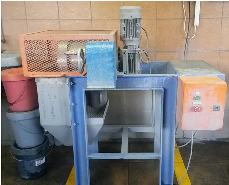
Figure 4-1: Laboratory Mill Rig
