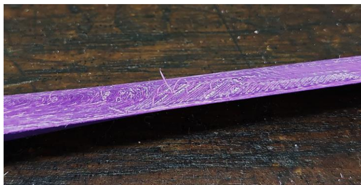
Figure 10. Test blade that was smoothed with ethyl acetate
