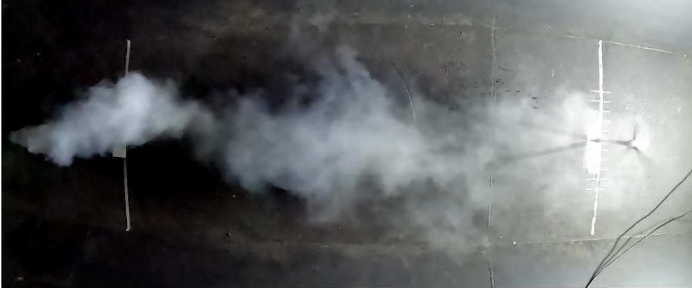
Figure 22. Screenshot of smoke visualisation of the wake from a video recording
