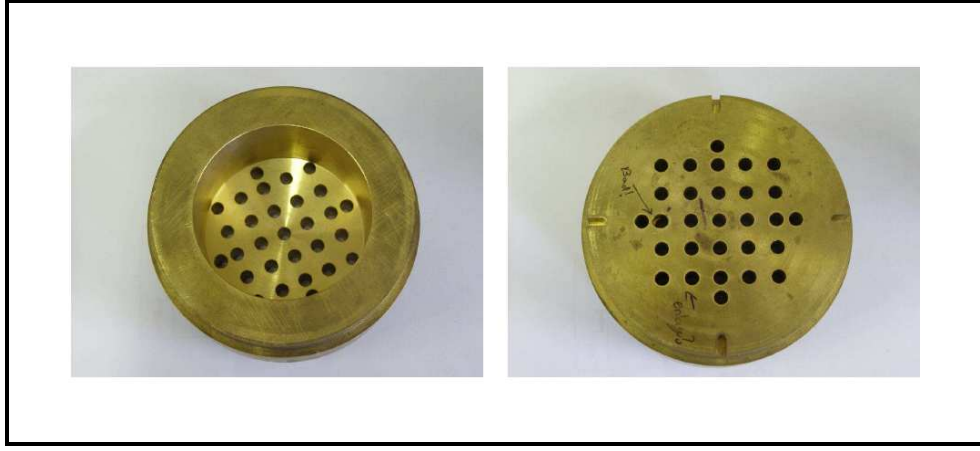
Figure 3.21: The pepper-pot collimator. This collimator has the following properties: its first hole from the middle on the x -axis/ y -axis is at 0.819^\circ (14.3 mrad), the second is at 1.679^\circ (29.3 mrad) and the third is at 2.251^\circ (39.3 mrad). The holes span 0.41^\circ (7.15 mrad), except for the smaller hole which spans \sim 0.20^\circ (3.57 mrad). The smaller hole, achieved by adding an insert, is not shown.
