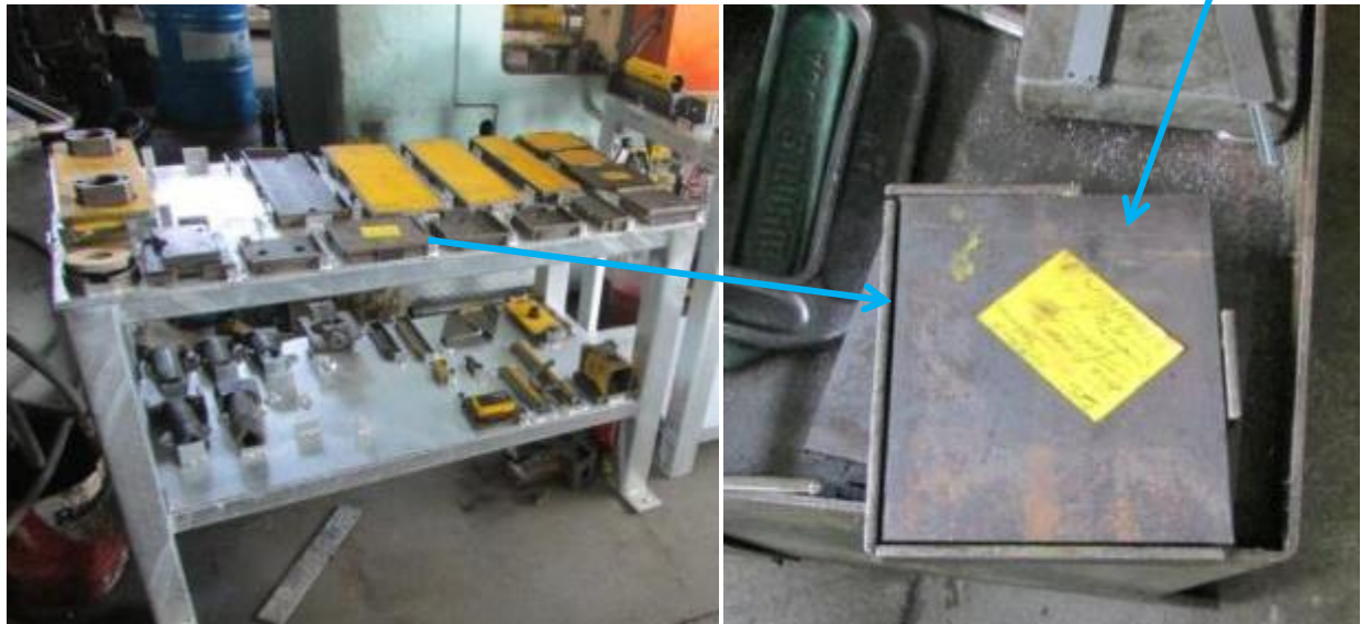
Figure 29: Checking Fixtures (Laursens2013)
