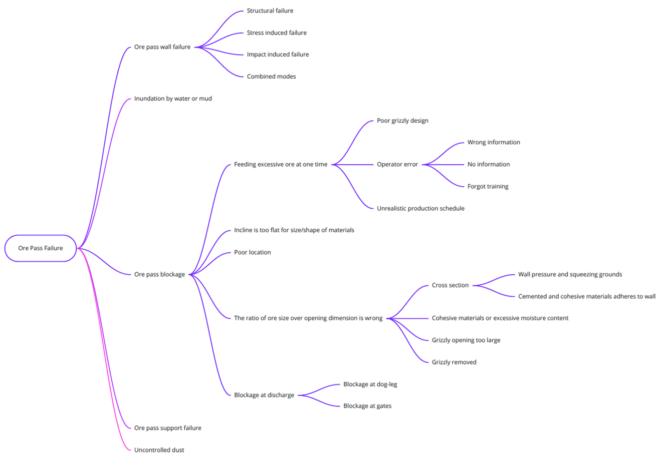
Fig. 12 A partial fault-tree diagram showing the main mechanisms of failure in ore passes (Adopted and modified from Beus et al. 1997)
