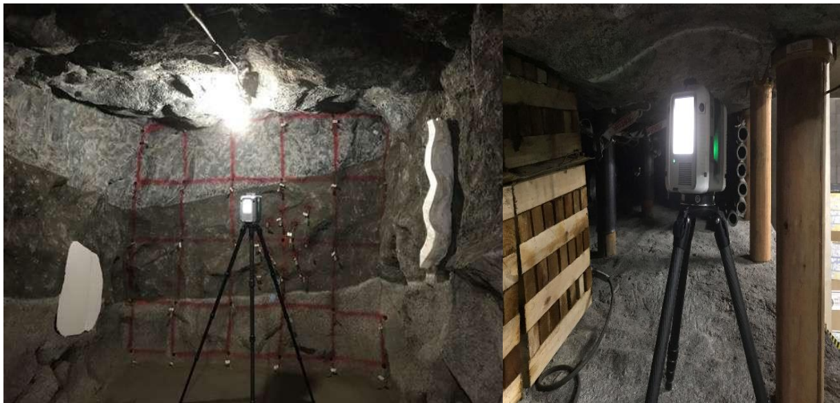
Figure 12: The static tripod mounted terrestrial laser scanner used was the RTC 360
