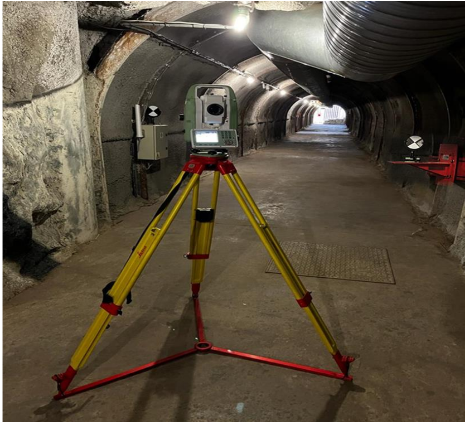
Figure 14: Total station and target set up to determine the coordinates and height of the three tie points.
