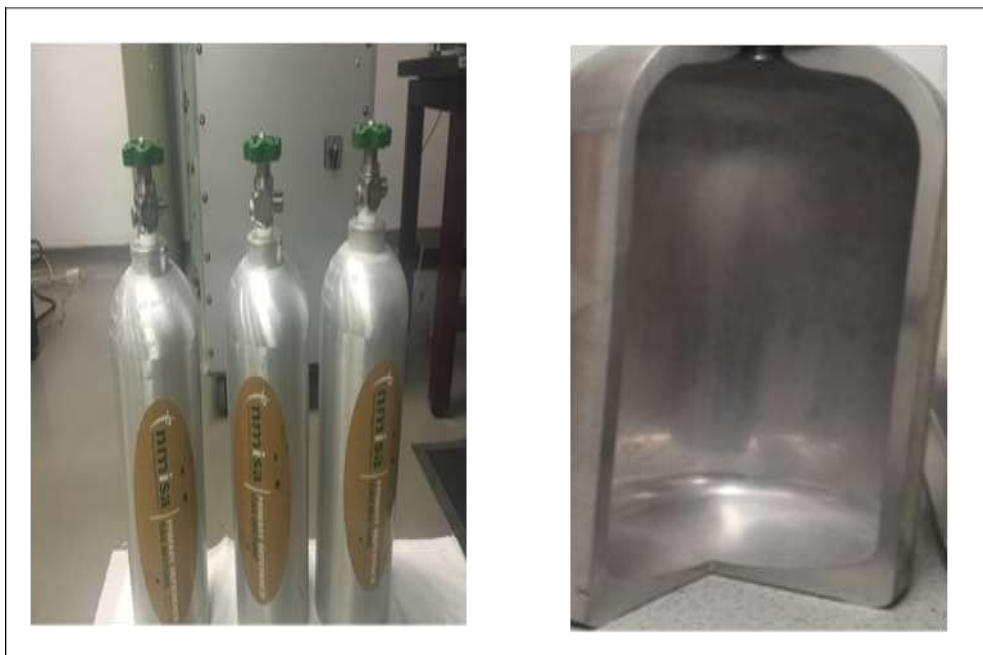
Figure 2.4. Demonstration of the inner components of a cylinder valve, the smooth inner walls of an aluminium gas cylinder.
