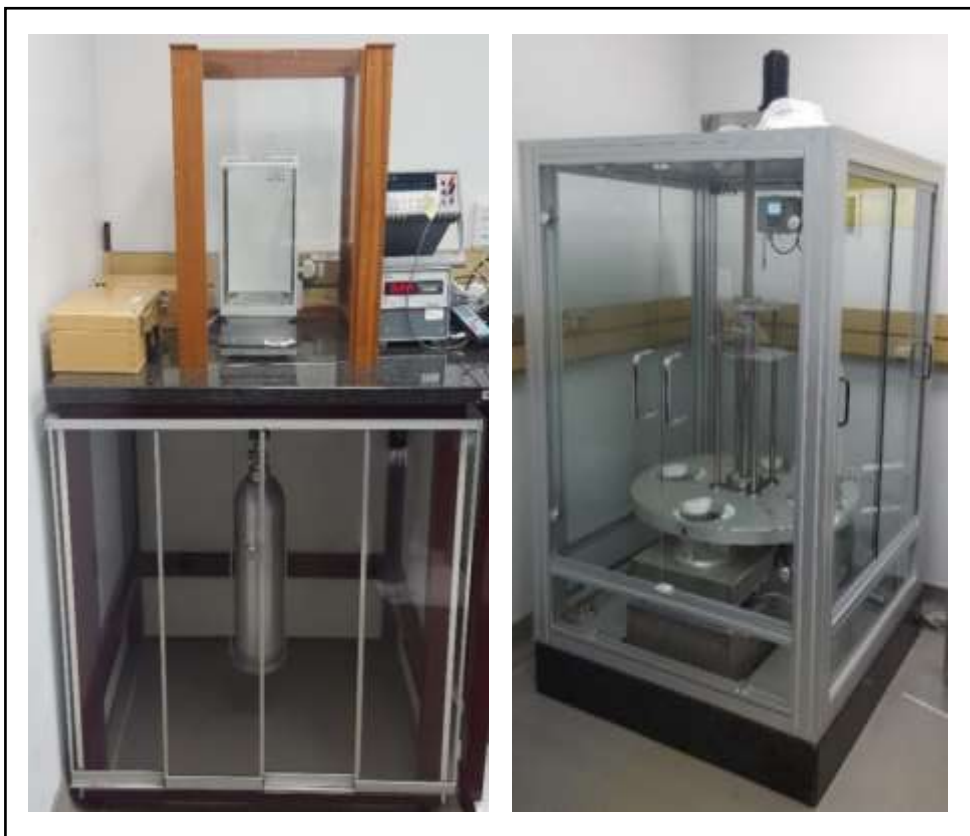
Figure 2.5. (a) Single-pan balance with 5 L cylinder suspended below, (b) Automated weighing system with a cylinder circular turntable plate by KRISS (Park et al, 2004).
