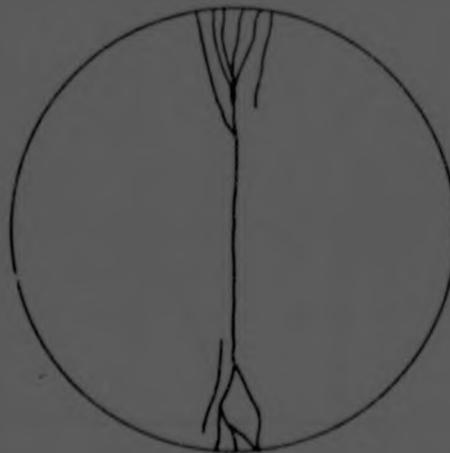
FIGURE B.2 TYPICAL FRACTURES RESULTING FROM LOADING SHOWN IN FIG B.1
