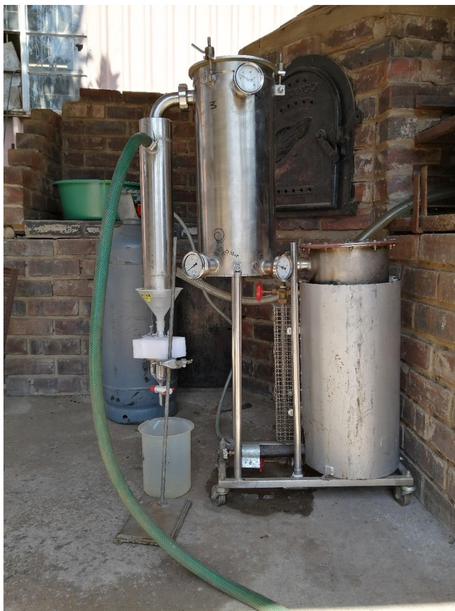
Figure 3.6. Gas-powered essential oil steam distillation unit in operation
