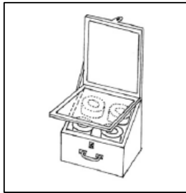
Figure 2.2 Schematic diagram of a box cooker (Panwar et al. , 2012)
