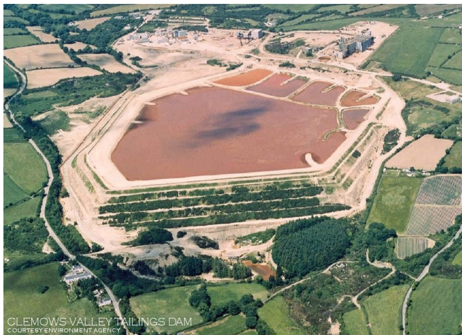
Figure 5: A typical tailings storage facility, Clemows Valley Tailings Dam ( http://www.cantabkent.co.uk/projectphotos/image_clemows.jpg )
