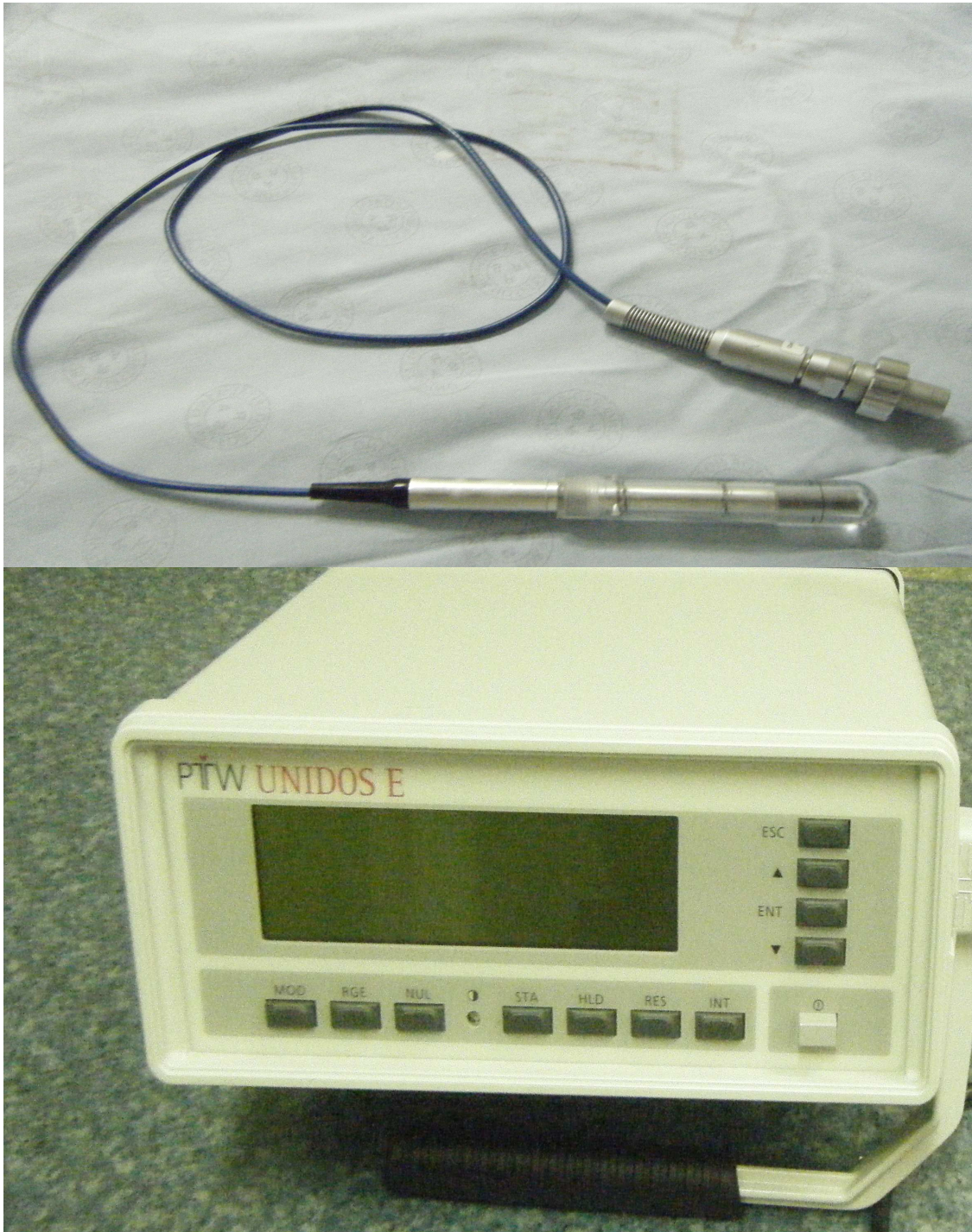
Figure 2.1 A thimble (0.6 cc Farmer-type) ionization chamber with build-up cap (top) and the PTW UNIDOS E electrometer (bottom).
