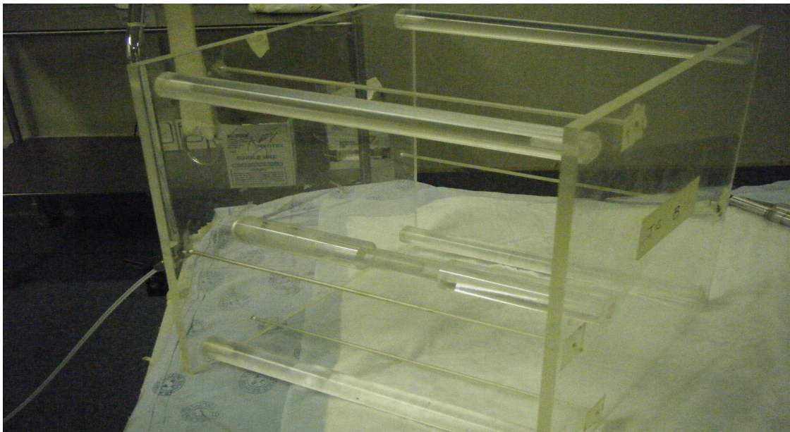
Figure 2.6 A Jig made of low density plastic. Its designed is such that it minimizes radiation scatter and positional uncertainty. It was used to hold the 0.6 cm 3 chamber and the radioactive brachytherapy source in fixed positions during measurements.
