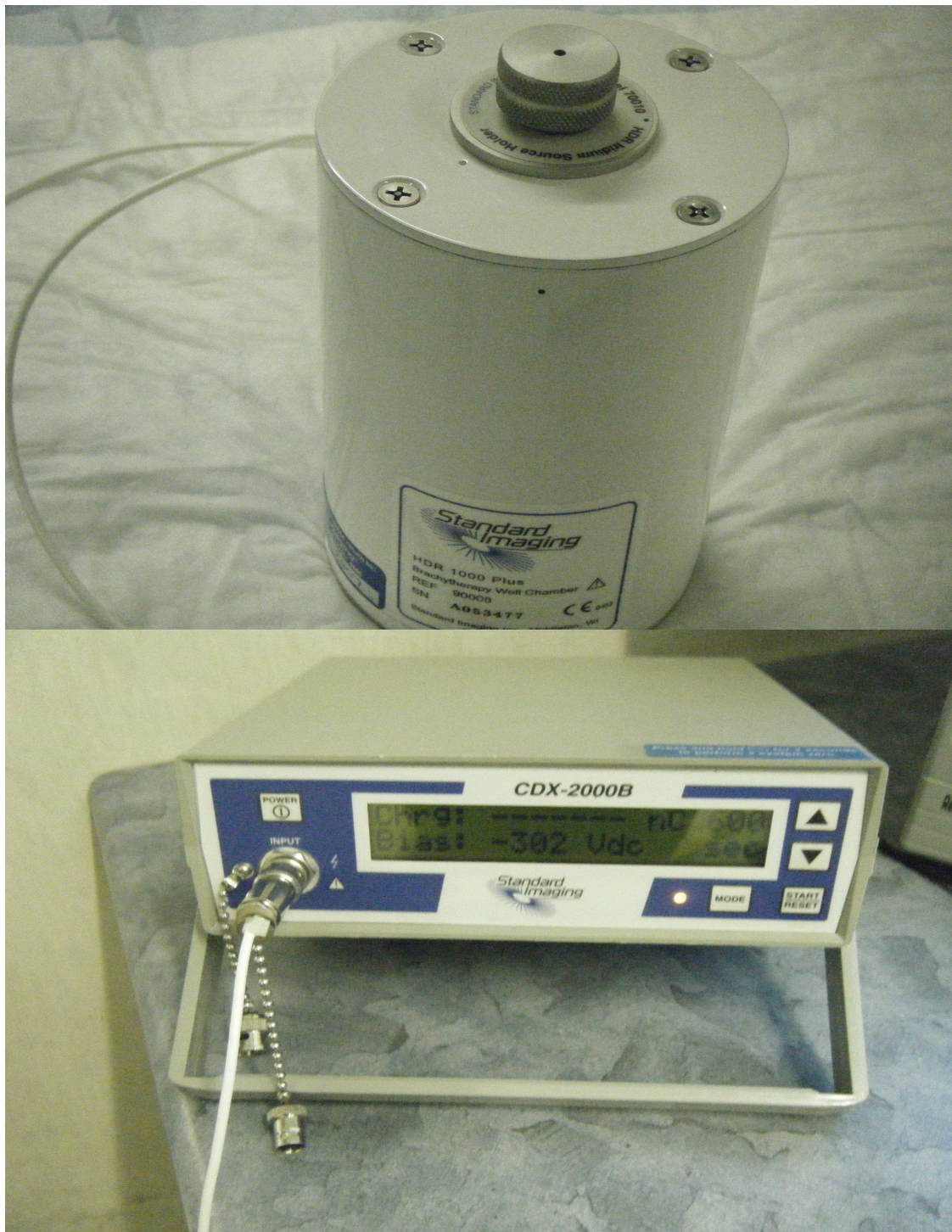
Figure 2.2 A Standard Imaging HDR 1000 Plus Brachytherapy well-type ionization Chamber (top) and the CDX-2000B Standard Imaging Electrometer (bottom).
