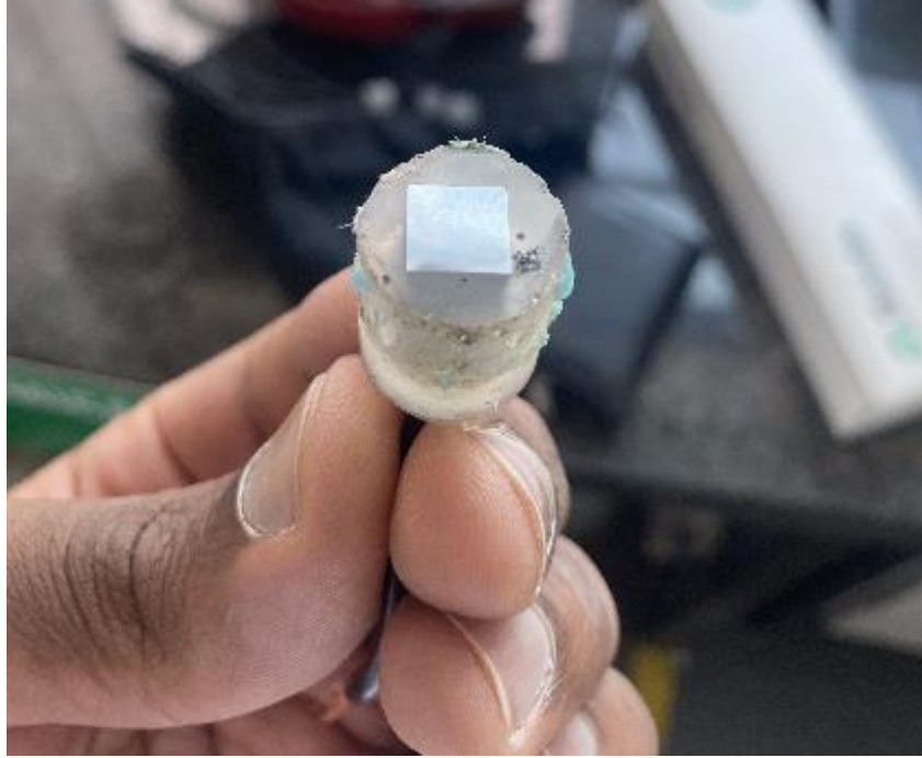
Figure 13: Mounted titanium sample in resin.
