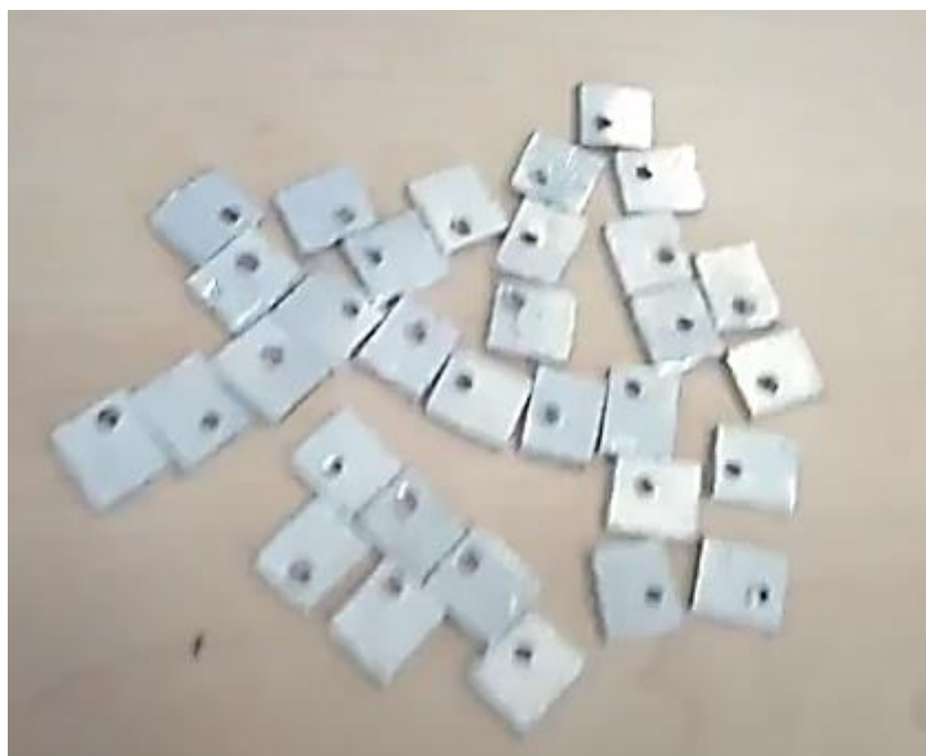
Figure 15: Prepared aluminium samples for weight loss test.
