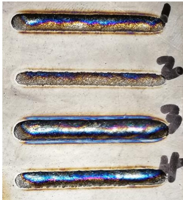
Figure 4.1: Single clads of Ti-Ni alloy, sample 1 produced at 600w with 0.5m/min, (2) at 600w with 1m/min, (3) at 1000w with 0.5m/min and (4) produced at 1000w with 1m/min.
