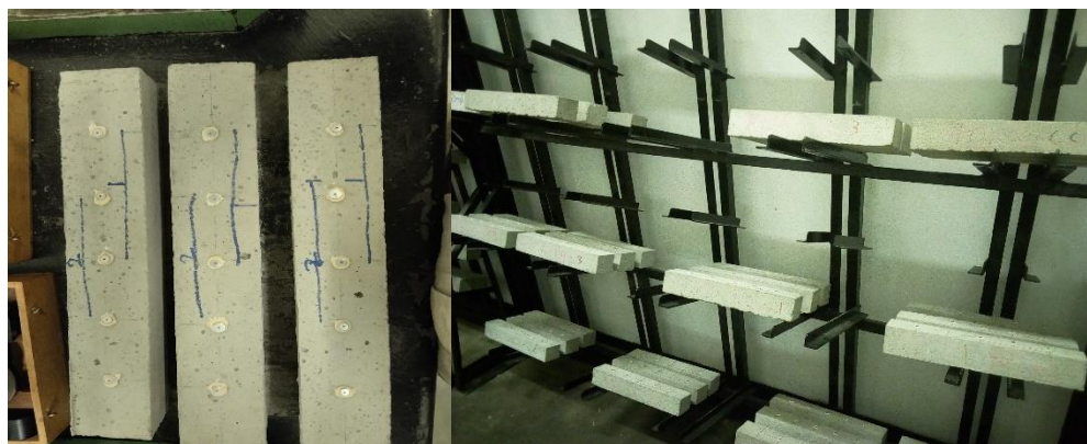
Figure 3.3: Drying shrinkage samples with stud arrangement and placement on steel rack
