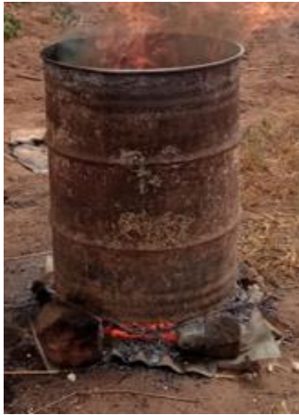
Figure 3.1: Drum furnace for the calcination of the corn cob
