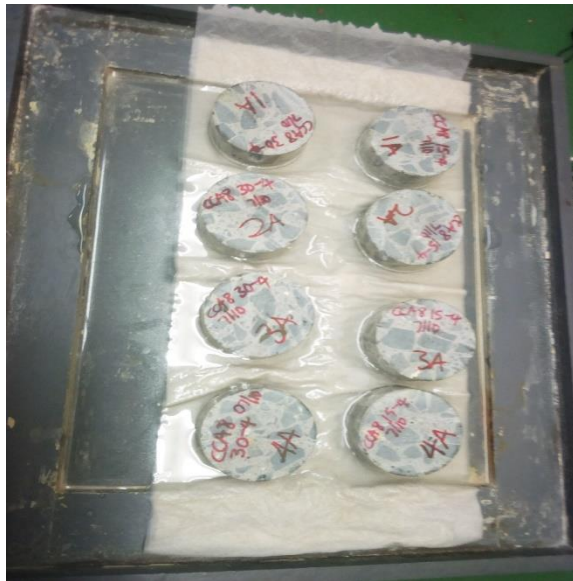
Figure 3.7: Testing of concrete cores for water sorptivity determination
